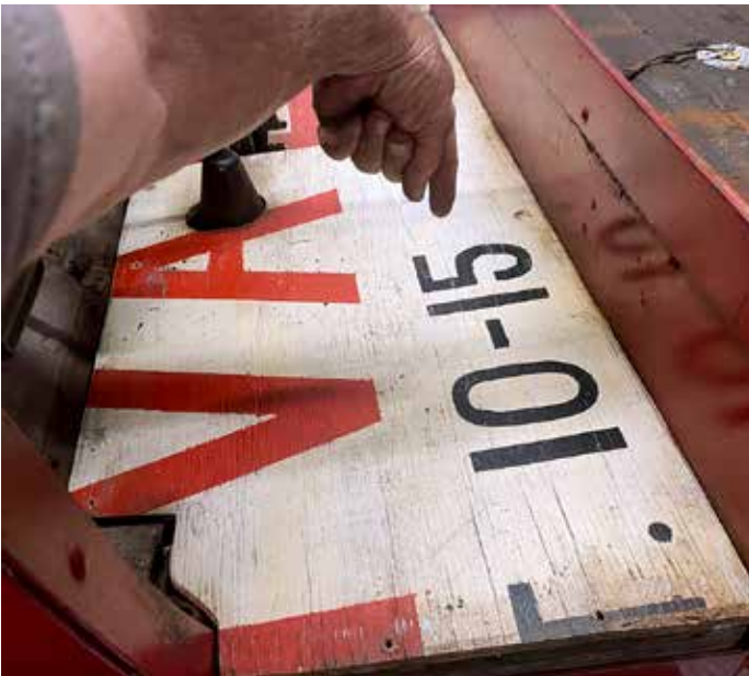
The hand is pointing to the spot where the master cylinder is located under the plywood. Obviously, there is no access to the master cylinder.
