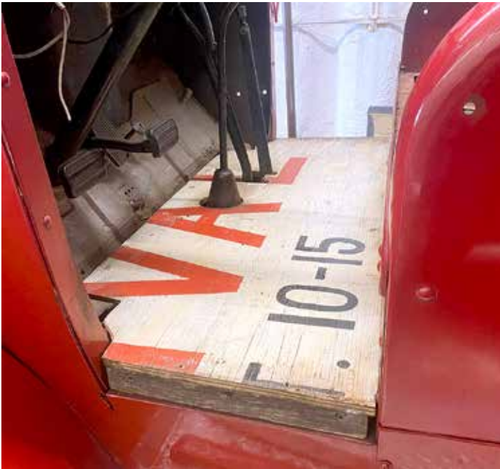
The plywood replacement floor board after removing the rubber matting and some metal trim.
