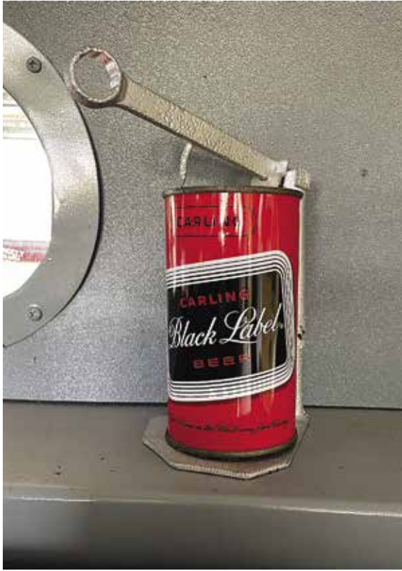
This homemade opener was made from a flat piece of steel welded to a hood latch. The end of a beer can opener and a nail were welded to a combination wrench that pivoted on the hood latch. This provided the 2 holes required in the steel cans of the day.
