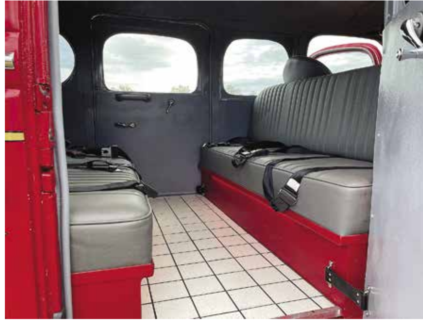
Remnants of the original headliner were fabric. I used ABS plastic and vinyl upholstery to make the interior. All photos by Mike Sanders.
