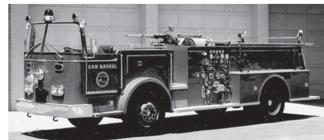
More than a year after the first one for Mountain View, the second Van Pelt Custom 300, serial #1512, was sold and delivered for $33,216.56 to San Rafael (CA) on June 7, 1961. It was the first to use Van Pelt's own factory-built chassis frame. The front siren was mounted higher and it had no compartments above the rear fenders. Van Pelt factory delivery photo from Lynn Chappell collection.
