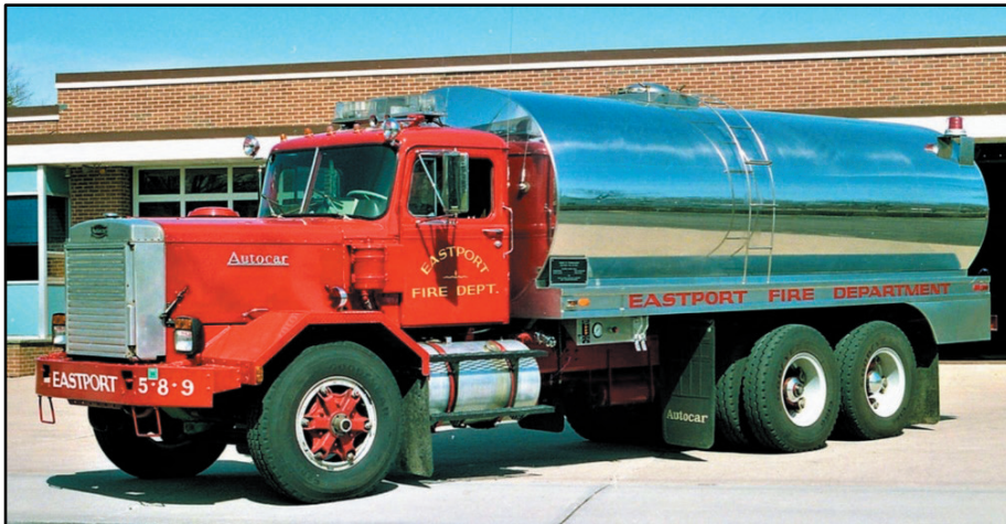
Garsite built this massive 4200-gallon tanker on a 1978 Autocar chassis for the Eastport Fire Department in Suffolk County.
