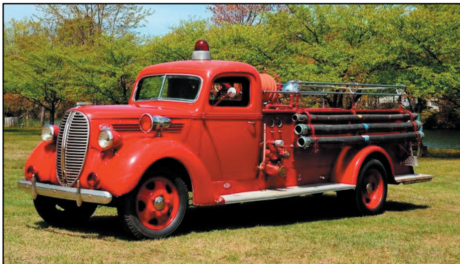
This 1938 Cayasler pumper was built on a Ford chassis with a 500-gpm pump and a 150-gwt. It served in North Branch, New York.
