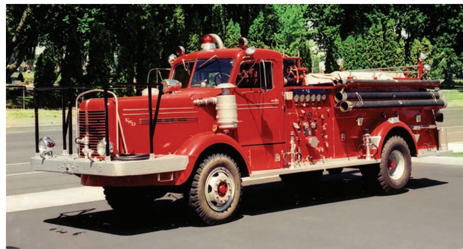
Walla Walla (WA) was running this 1953 FWD pumper as Reserve Engine 1 when Mr. Hattersley took this photo. It is equipped with a 750-gpm pump and a 550-gwt. Note the front bumper is set-up to have personnel ride for brush fires.
