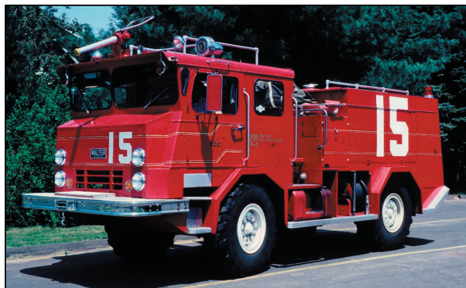
Among the many not-so-well-known fire apparatus builders in New York State was Garsite Products, Inc., of Long Island, which built this unique 1967 industrial pumper on a Walter 4x4 chassis.
