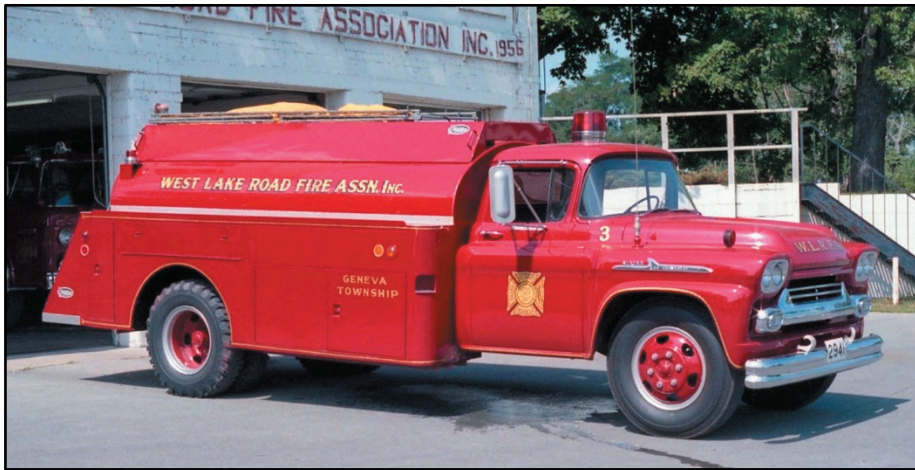
The Kaustine Furnace and Tank Company built this 1500-gallon tanker for the West Lake Road Fire Association on a 1958 Chevrolet chassis.
