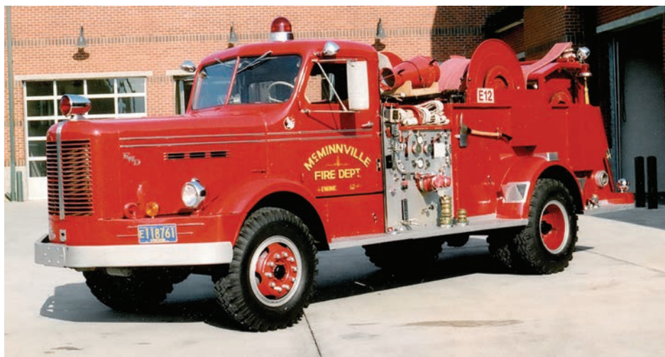
McMinnville (OR) Fire Department's Engine 12, a 1952 FWD pumper. This rig has a 1,000-gpm pump, 80 gallons of foam, and a reel with 1,300-feet of 5-inch hose in the rear.
