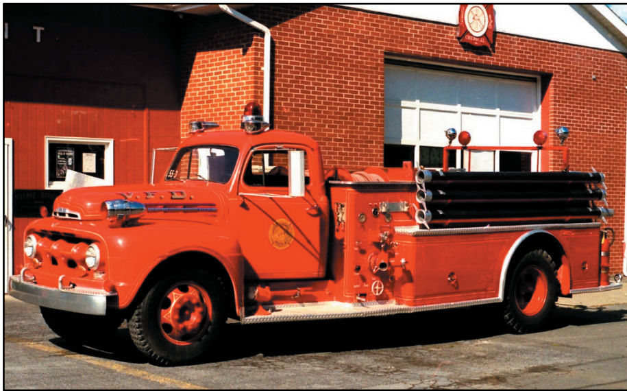
The Valatie Fire Department in Columbia County operated this 500-gpm triple combination pumper that was built by Ribley and Harpinger.
