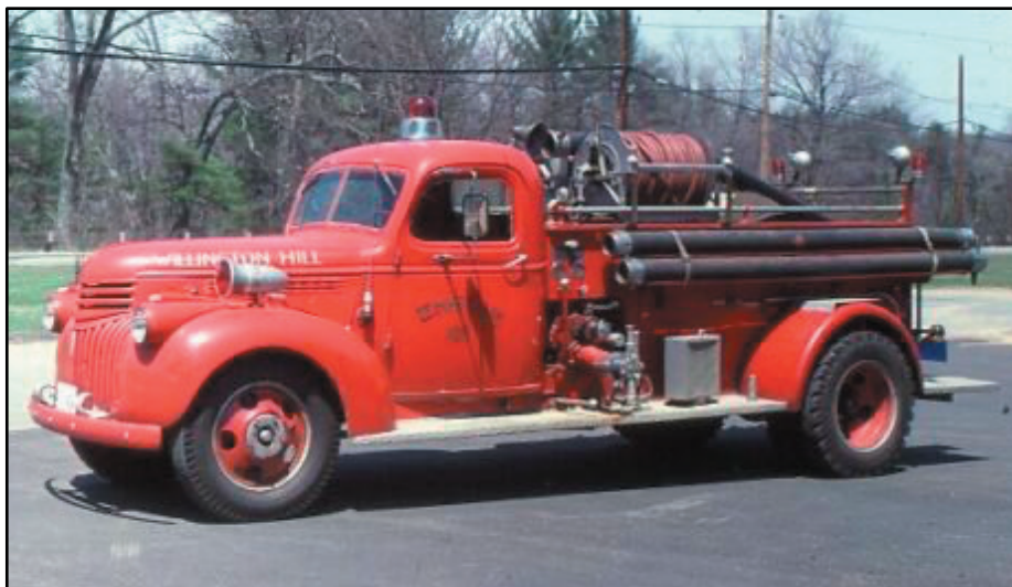
Cayasler built this 500-gpm pumper on a Chevrolet chassis for the U.S. Army in 1943. It later served in Willington Hill, Connecticut.
