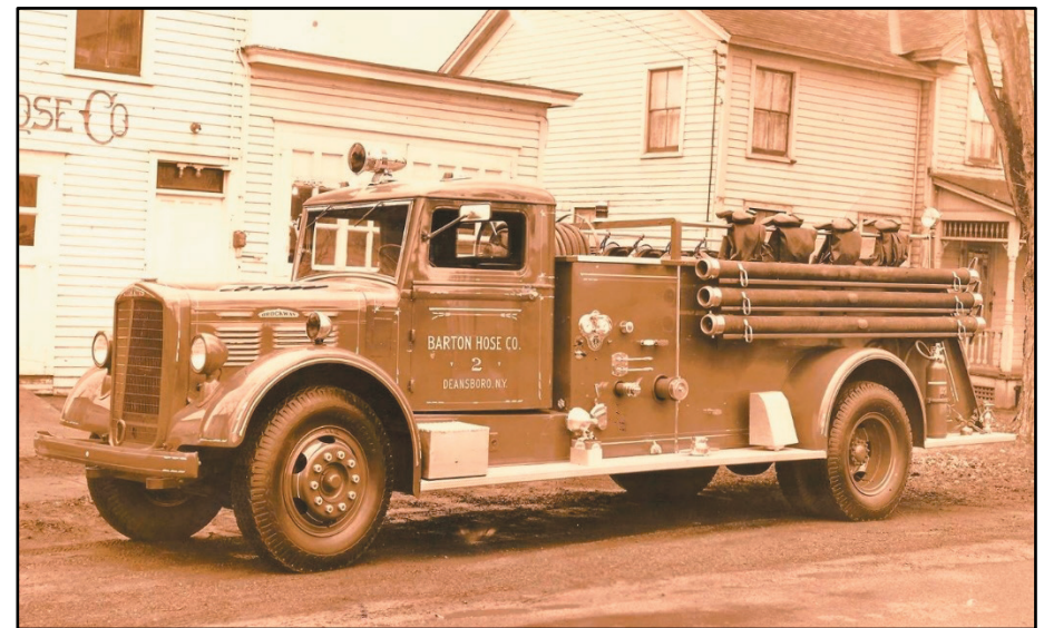
The Fire Apparatus Engineering Corporation of Clayton built this pumper on a Brockway truck chassis for the fire department in Deansboro, New York.
