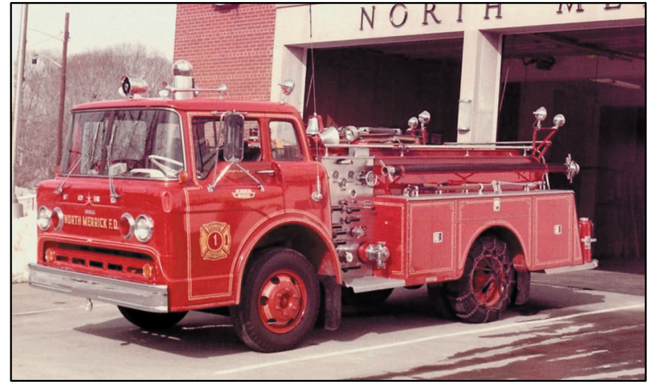
The North Merrick Fire Department in the Town of Hempstead, Nassau County, operated this compact 1962 Garsite 500-gpm pumper that was built on a Ford C-600 chassis.
