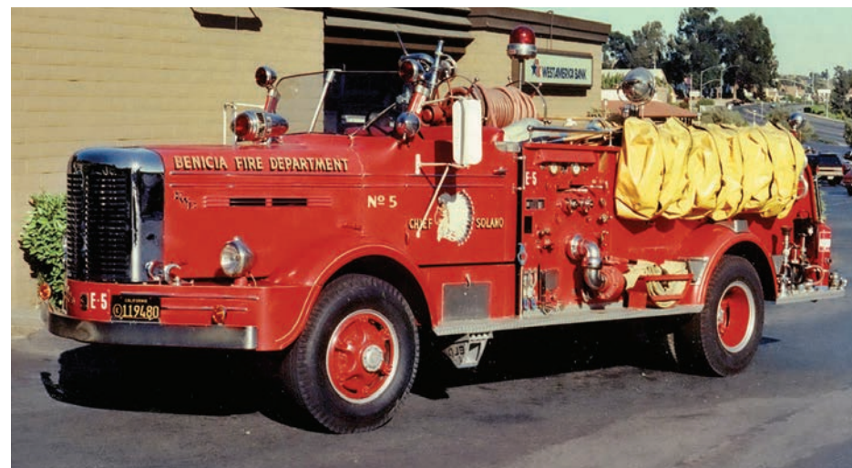
This 1949 FWD was in service for the Benicia (CA) Fire Department as Reserve Engine 5 when this photo was taken. The pumper has a 1,250-gpm pump and 500-gwt.
