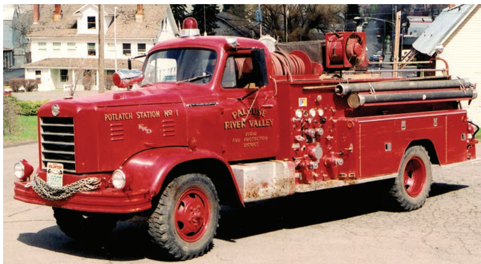
Potlatch (ID) Fire Department's Engine 1. This 1956 FWD pumper has a 750-gpm pump and 550-gwt.
