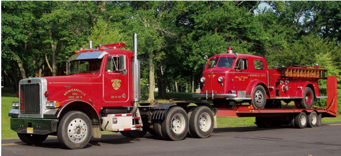
The New Jersey Fire Museum uses this 1989 Peterbilt tractor that formerly pulled a water tanker for the Morganville (NJ) fire department and was transporting a 1947 American LaFrance 1000-gpm pumper that formerly served Milltown (NJ).
