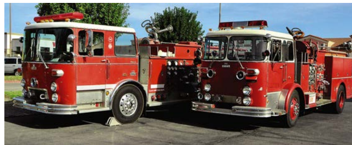
On the left is Dave Kromka's 1975 Crown pumper (ex-Culver City, CA) is equipped with a 1,500-gpm pump and had a 500-gwt. On the right is Dan Page's 1975 Crown pumper (ex-Upland, CA Fire Department) is equipped with a 1,500-gpm pump and had a 500-gwt.
