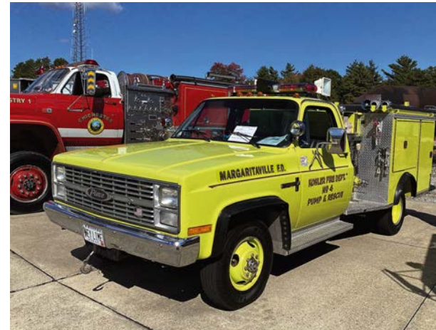
Ray Smith's 1984 Chevrolet K30 4x4 Pierce Mini-pumper, "Margaritaville FD" 400-gpm pump and a 250-gwt. on display at the AREC Muster.
