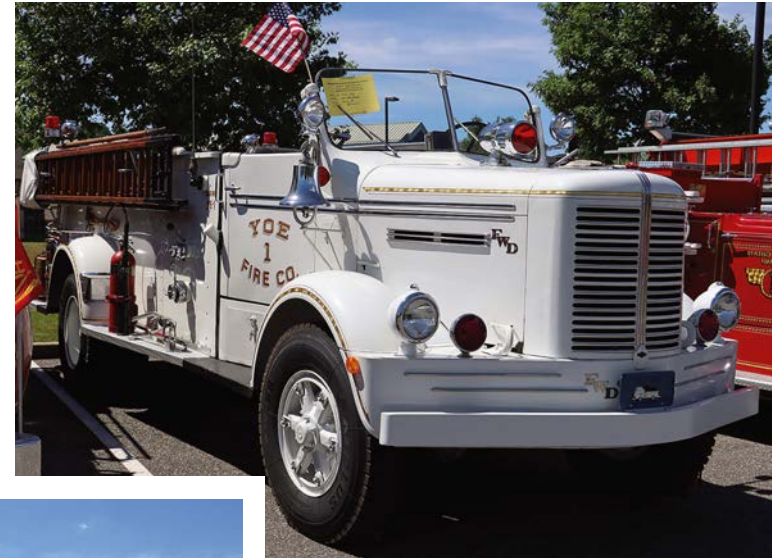
1951 FWD pumper with a 500-gpm pump. Photo by Tommy Herman.
