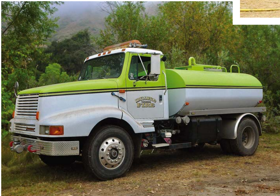
This Water Tender is built on an International chassis. The rig is ex-Idyllwild (CA) Fire Department. All photos by Kent Collum.
