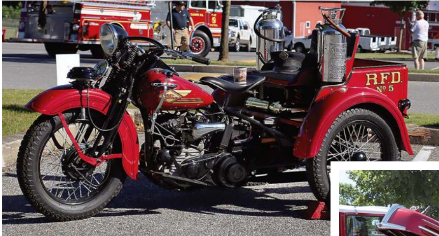
1935 Harley-Davidson Firecycle, one of ten used by the Richmond (VA) Fire Department. The motorcycles equipped with sidecars carried 150 to 250' of 1/2" rubber hose, two portable extinguishers, axe, plaster hook, Johnson pump and bucket, wire brooms, etc. Photo by Tommy Herman.
