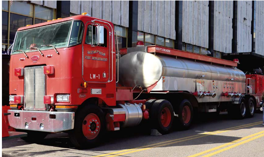
The Fire Museum of Memphis owns this Foam Rig. It responded as Light Water 1. The trailer carried 4,000 gals of Alcohol Type Foam and was built in 1980 by FM Chemical Company in Ontario, CA. A Peterbilt tractor still pulls the rig.
