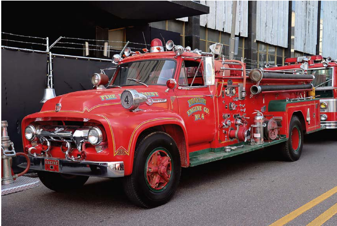
1954 Ford/Oren 750-gpm pumper (ex-Braxton, MS). Note the green running boards.
