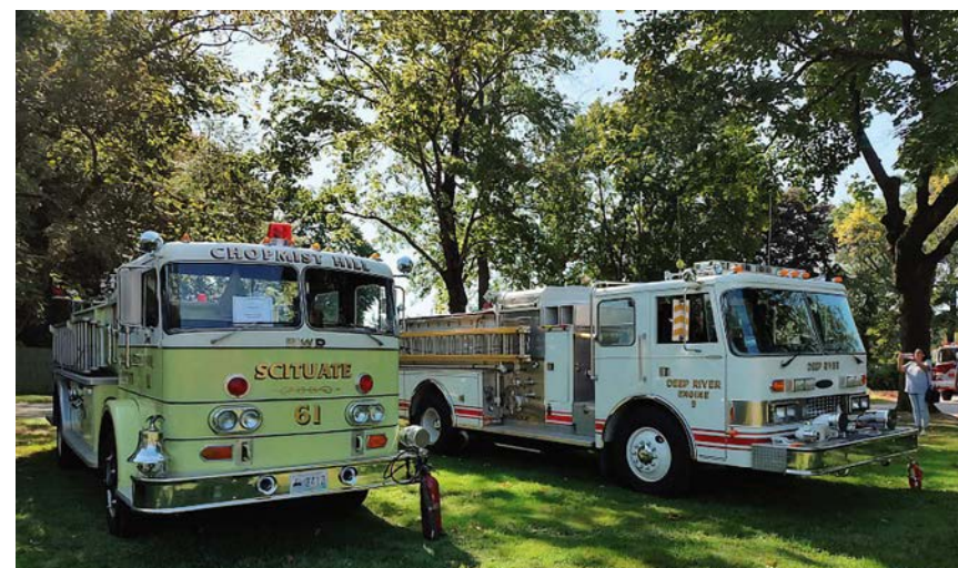
On the left is a 1963 FWD/Farrar pumper (ex-Scituate, RI) and currently owned by the Chopmist Hill Volunteer Fire Department. On the right is a 1983 Pierce Dash pumper (ex-Deep River Fire Department in Connecticut). The Pierce has a 1,250-gpm Waterous pump and a 750-gallon tank. The rig served from 1983 until July of 2023 and had been in reserve for over 20 years. The Pierce was purchased from the department in November of 2023 by its second and present owners, Ernesto Cabral and Jed Barton.
