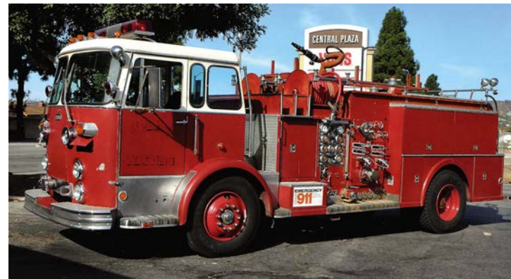
Dan Page own this 1975 Crown pumper (ex-Upland, CA) equipped with a 1,500-gpm pump and 500-gwt. Photos by Kent Collum.
