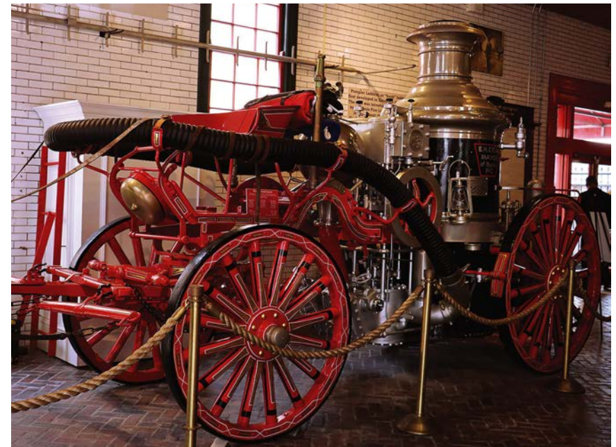
1910 Ahrens Continental 900-gpm steam fire engine. The rig was named for Memphis Mayor E. H. Crump.
