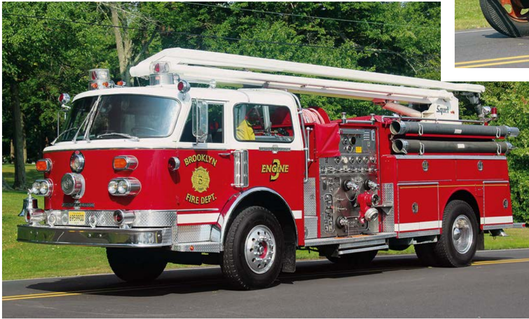
Former Brooklyn (OH) Engine 3 a, 1981 American LaFrance 1,000-gpm pumper with a 300-gallon tank and 54-foot Squirt.
