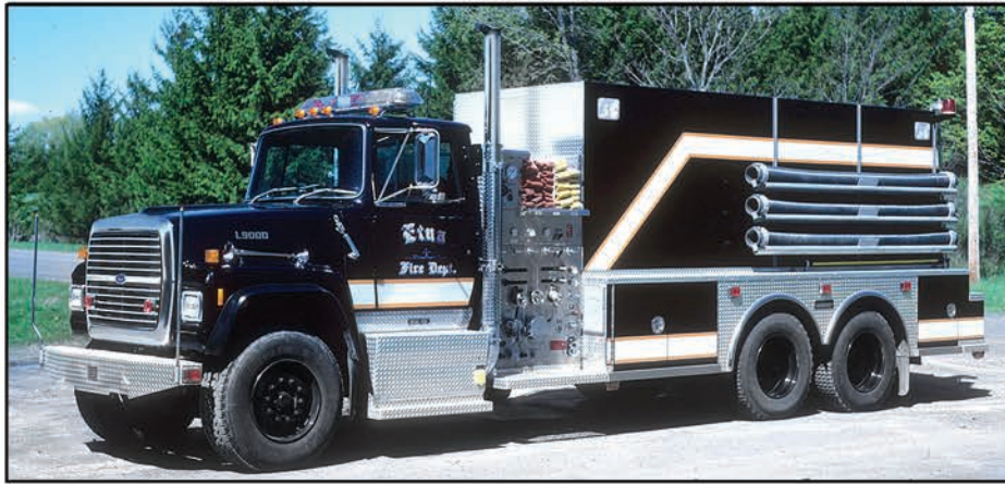
The Etna Fire Department in Tompkins County, New York, operated this 1993 Saulsbury 2,500-gallon tanker, that was built on a Ford L-9000 chassis with a 1,500-gpm pump.
