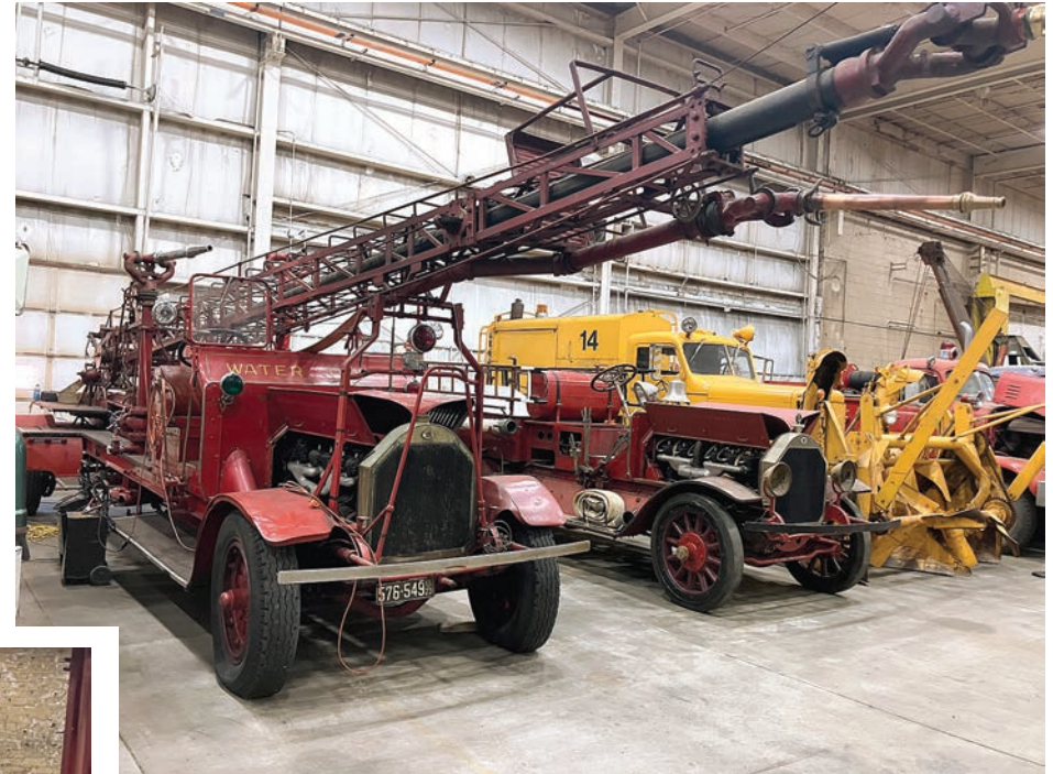
1923 Seagrave water tower with rear-mounted 65' mast, one of three delivered to Chicago Fire Department. This rig ran as Water Tower No. 3.
