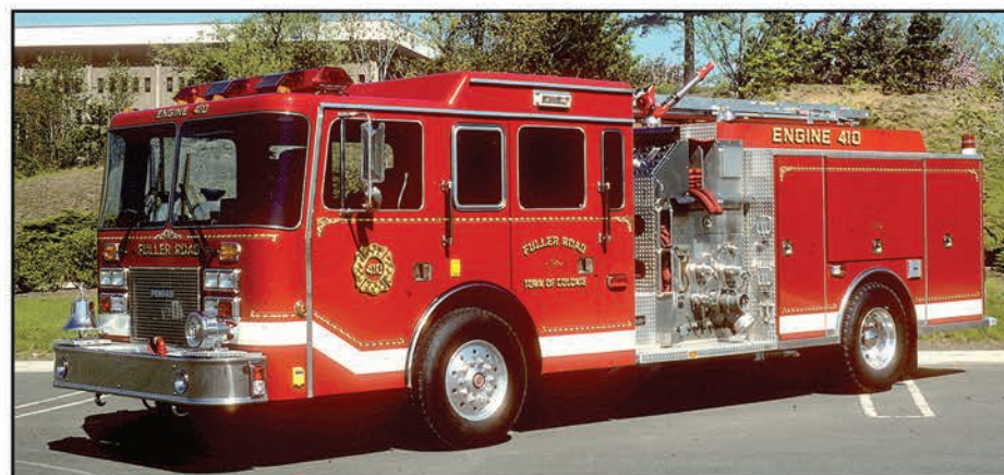
The Fuller Road Fire Company in the Town of Colonie, Albany County, New York, operated this 1993 Saulsbury 2,000-gpm pumper that was built on a Pemfab chassis. It had an extended cab and a 500-gwt.
