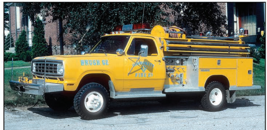
The Community Fire Company in Seven Valleys, Pennsylvania, operated this 1976 Saulsbury mini-pumper that was built on a Dodge 4x4 chassis. It had a 250-gpm pump and a 200-gwt.
