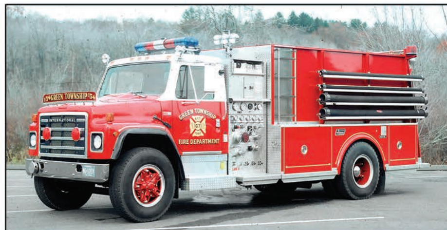
This 1984 Saulsbury tanker served in Green Township, New Jersey. It was built on an International chassis with a 750-gpm pump and a 2,000-gwt, which was about the most water that could be carried safely on a single rear axle.
