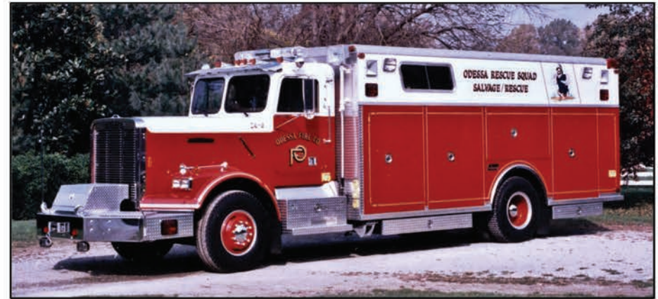
Sixty miles north of Seaford, is Odessa, Delaware, where this 1986 Saulsbury walk-in rescue served. It was built on a conventional Freightliner chassis. It was retired in 2007. It replaced a 1974 Saulsbury walk-in rescue that was built on a Ford C Series chassis.
