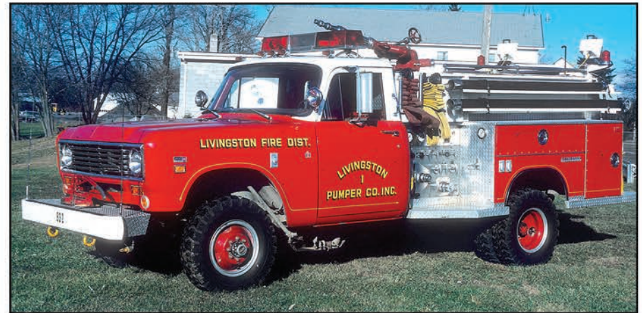
Before building full-size pumpers, Saulsbury built many mini-pumpers, such as this 1975 unit on an International chassis for Livingston in Columbia County, New York. It had a 350-gpm pump and a 275-gwt.
