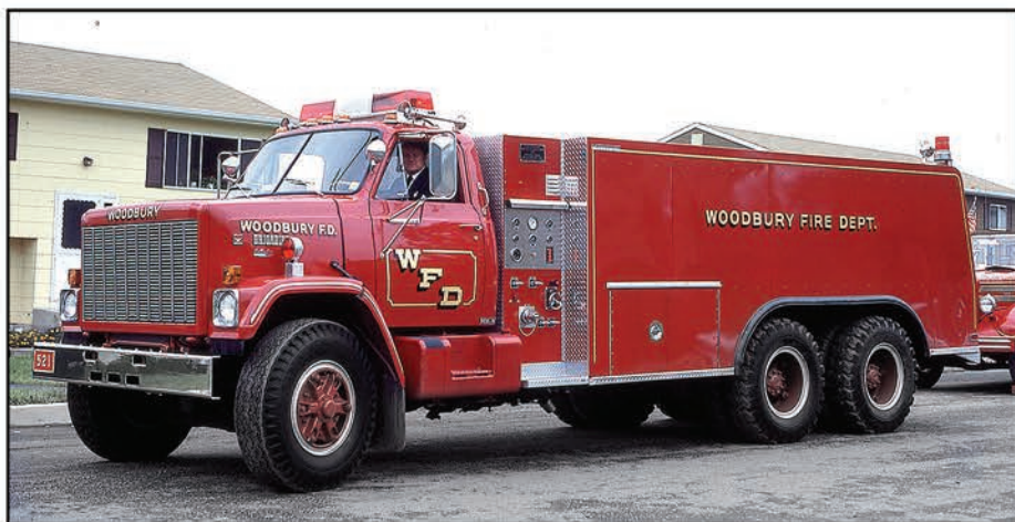
Saulsbury built this 3,500-gallon flat side tanker for the fire department in Woodbury, Orange County, New York, on a 1979 Chevrolet Brigadier chassis. It had a 400-gpm pump.
