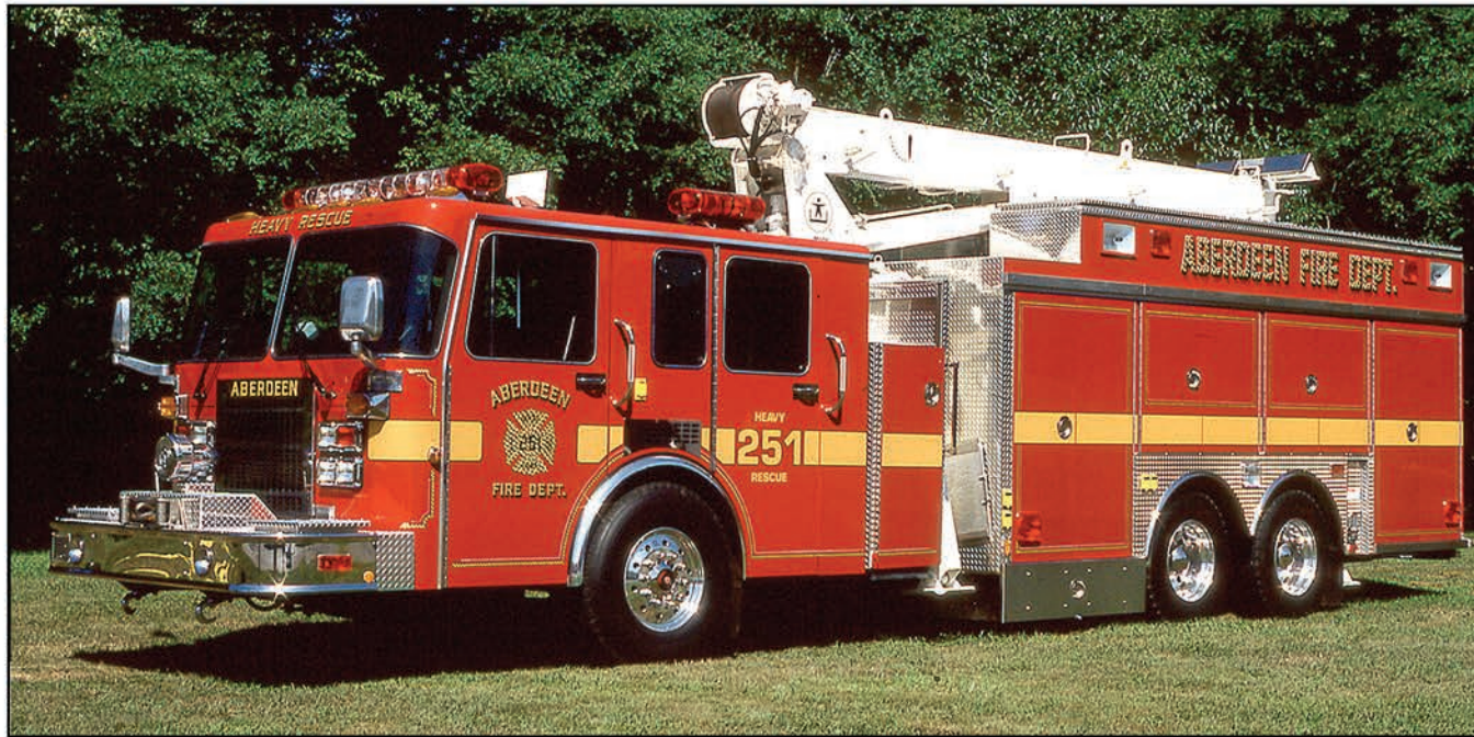
Among the more impressive heavy rescue trucks built by Saulsbury was this one, which was built in 1993 on a tandem axle Spartan chassis. It is equipped with a 57-foot 14-ton JLG crane. It serves with the Aberdeen Fire Department in Harford County, Maryland. Its first due area includes Interstate 95.
