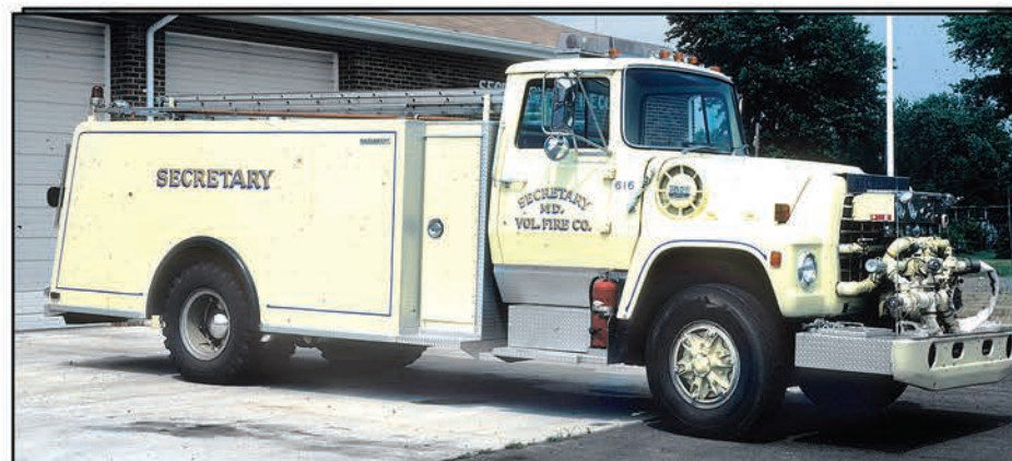
The Secretary Fire Volunteer Fire Company in Maryland operated this 1976 Saulsbury tanker that was built on a Ford Louisville Series chassis with a 750-gpm front mounted pump. John Floyd photo.
