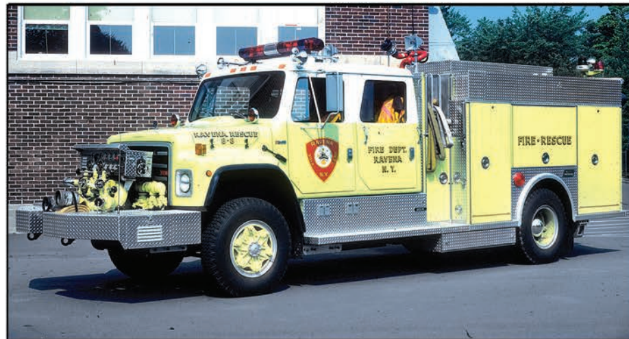
In 1983 Saulsbury built this interesting 4x4 rescue truck for Ravena in Albany County, New York. Rescue 8-8 was built on an International chassis with a 1,000-gpm front mounted pump and a 500-gwt.
