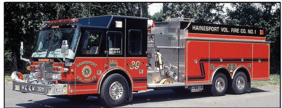
Saulsbury built this unit in 1995 on a Simon Duplex chassis with a 2,000-gpm pump and a 2,500-gwt for Hainesport, New Jersey. In 2014, Tender Engine 3911 was remounted by Pierce on an Arrow XT chassis.
