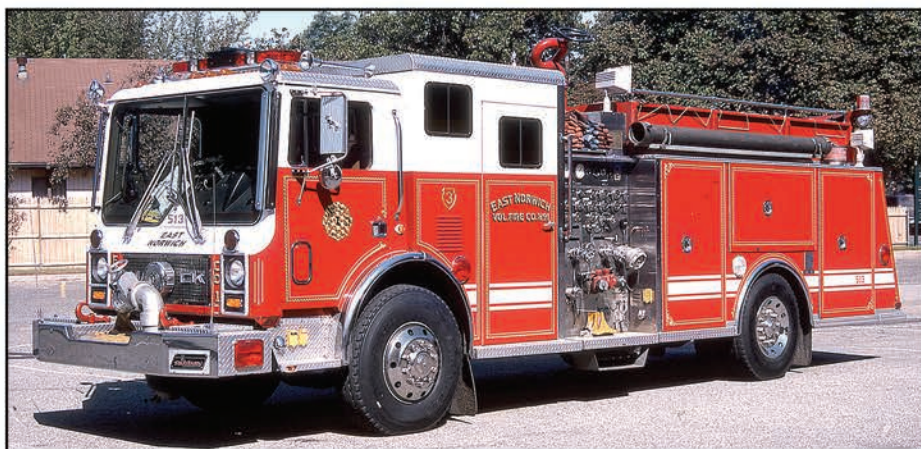
Four-door cabs still were not standard in 1987 when this Saulsbury triple combination pumper was delivered to East Norwich in Nassau County, New York. It had a 1,750-gpm pump and a 500-gwt. East Norwich operated several other Saulsbury apparatus.
