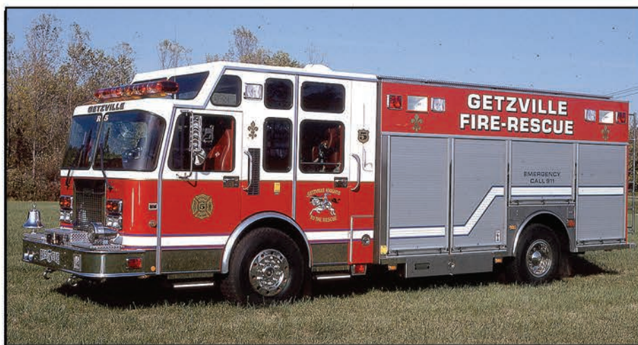
The Getzville Fire Department in Amherst, Erie County, New York, operated this 1997 Saulsbury walk-around rescue that was built on a Spartan chassis and featured a 16-inch raised roof on its cab.
