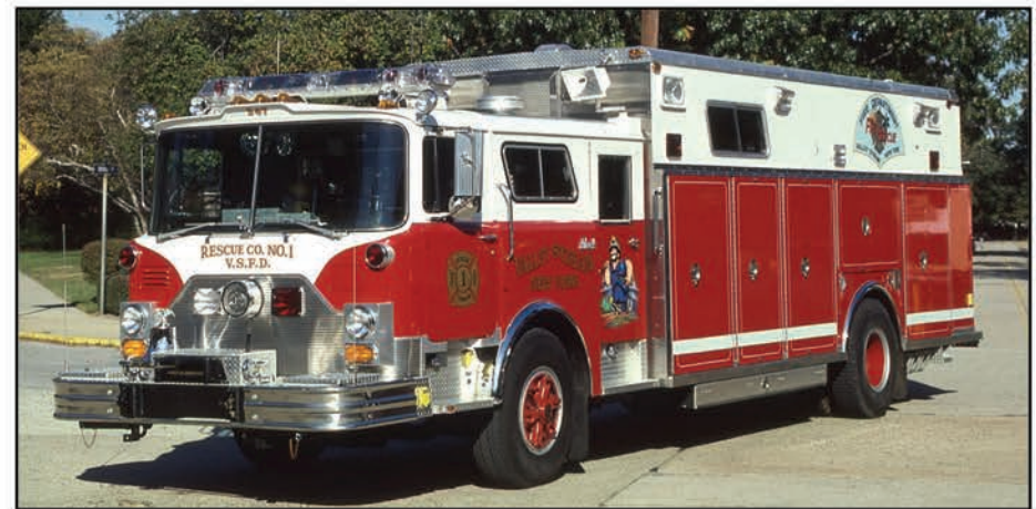
The Valley Stream Fire Department in Nassau County, New York, operated this 1987 Saulsbury walk-in rescue that was built on a Mack CF Chassis. It was part of an all Mack CF fleet with four engines, an LTI rear-mount aerial and an Aerialscope tower ladder.
