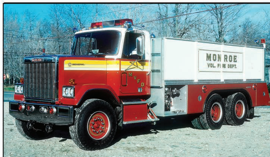
The fire department in Monroe, Connecticut, operated this 1979 Saulsbury tanker that was built on a GMC General tandem axle chassis. This had a 400-gpm pump and a 3,600-gwt.
