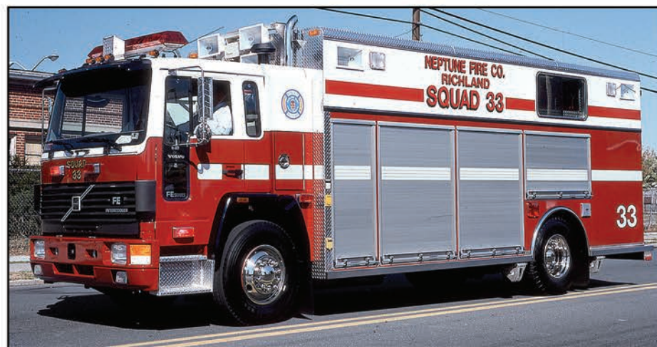
The Volvo FE was an unusual choice for fire apparatus. This one was used by Saulsbury in 1993 to build this walk-in rescue with roll up doors for the Neptune Fire Company in Richland, Pennsylvania.
