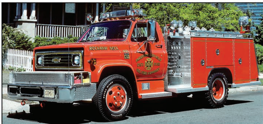
Somewhat overlooked by history is the “midi” pumper. The concept never gained any traction in the fire service. Parsippany, New Jersey, operated this 1976 Saulsbury “High Sierra” midi-pumper, which was built on a Chevrolet chassis. It had a 250-gpm pump and a 250-gwt.
