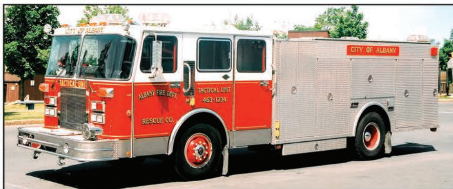
The Rescue Company in Albany, New York, operated this 1988 Saulsbury rescue. Built on a Spartan chassis, this rescue truck is notable for its diamond plate body, which was "spartan" in the truest sense of the word.
