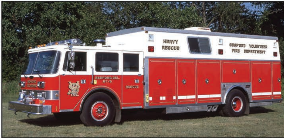
Seaford, Delaware, operated this heavy rescue that Saulsbury built on a 1986 Pierce Arrow chassis. The Arrow was introduced in 1979 and had an all-aluminum cab. It was the first custom chassis built entirely by Pierce.
