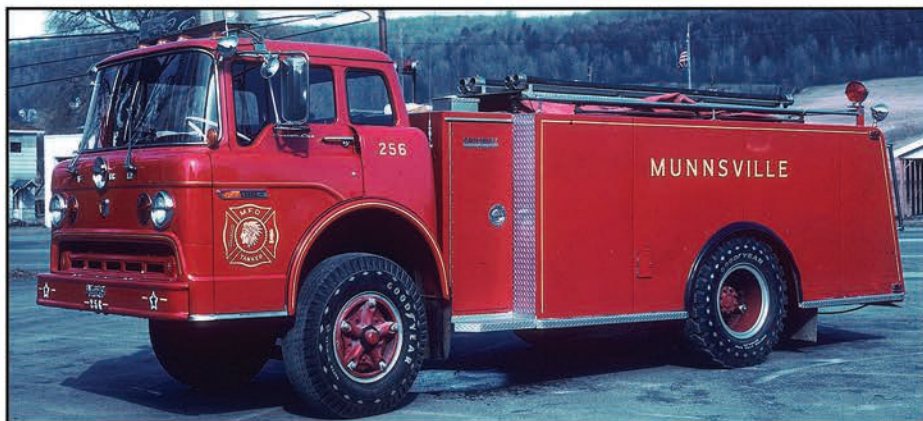
The Village of Munnsville in Madison County, New York, operated this 1972 Saulsbury tanker that was built on a Ford C-900 chassis with all-wheel drive.
