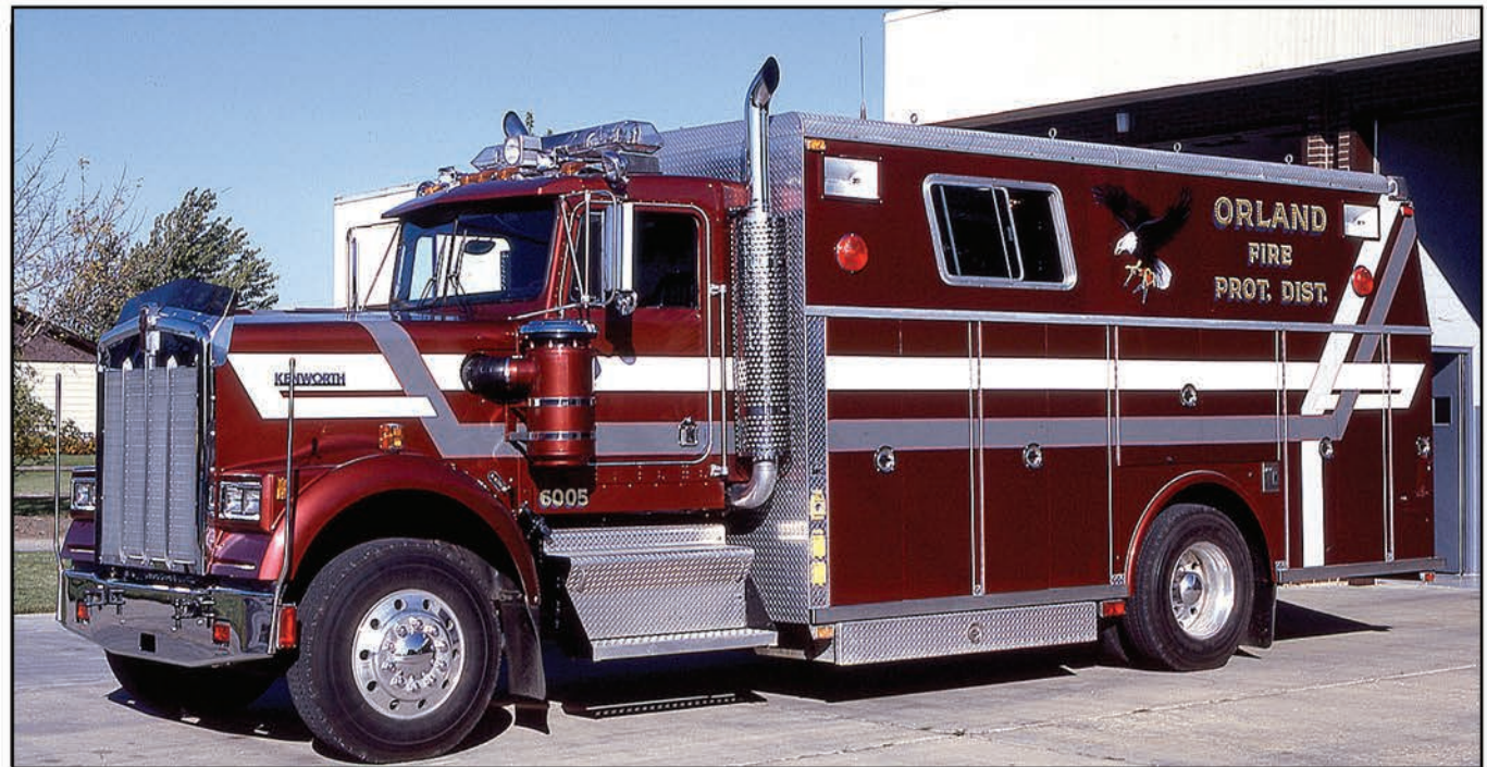
The Chicago suburb of Orland Park operated this 1998 Saulsbury walk-in rescue that was built on a Kenworth conventional chassis. Kenworth is a very unusual choice for fire apparatus as is the deep burgundy livery of this very muscular looking rescue truck.
