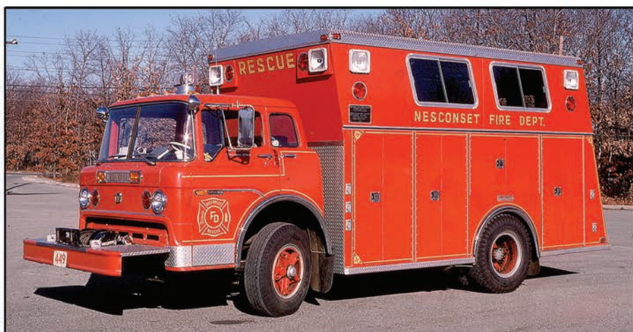
Saulsbury built its custom rescue trucks on many different types of commercial chassis. This 1971 walk-in rescue was built on Ford C-600 chassis for the Nesconset Fire Department in Suffolk County, New York. The Ford C was the most popular among Saulsbury's customers and the most popular across the fire service.
