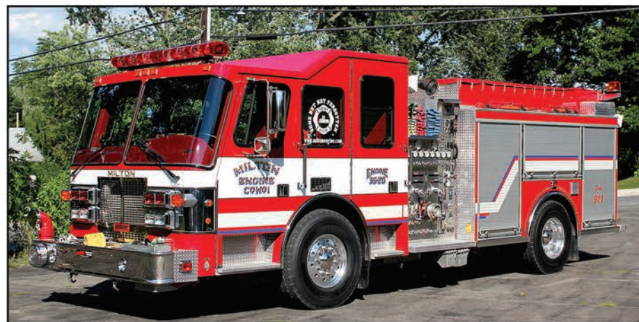
In the 1990s Saulsbury built many pumpers on Simon Duplex chassis, like this 1996 rescue pumper that was built for the Milton Engine Company in Ulster County, New York. It has a 2,000-gpm pump and a 900-gwt. It also carries 100 gallons of foam and extrication equipment.
