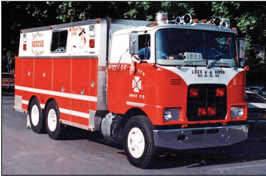
Saulsbury used a 1979 Mack F Series cab-over-engine chassis to build this tandem axle walk-in rescue truck for Lock Haven, Pennsylvania.
