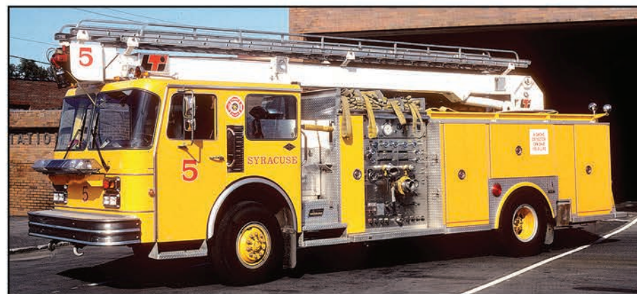
Syracuse, New York, operated this 1987 Spartan-Saulsbury “maxi” pumper with a 2,000-gpm pump a 500-gwt and a 55-foot LTI Fire Stix.
