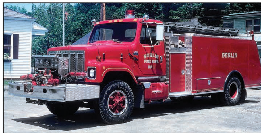
The Berlin Fire Department in Rensselaer County, New York, operated this 1981 Saulsbury Bison Series tanker built on an International chassis with a 1,000-gpm pump, a 1,600-gwt, an aluminum body and a rear quick dump.
