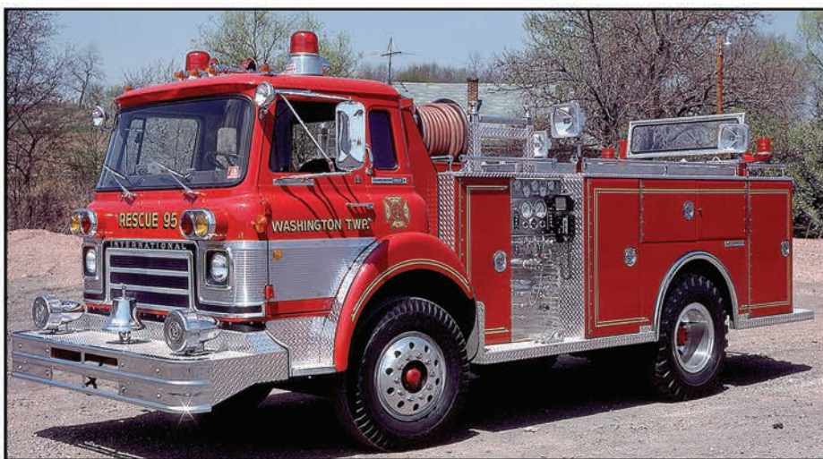
Two Federal Q sirens would be overkill for a full-size pumper, let alone this 1977 midi that was built on an International chassis for Washington Township, Pennsylvania, with a 500-gpm pump and a 500-gwt.
