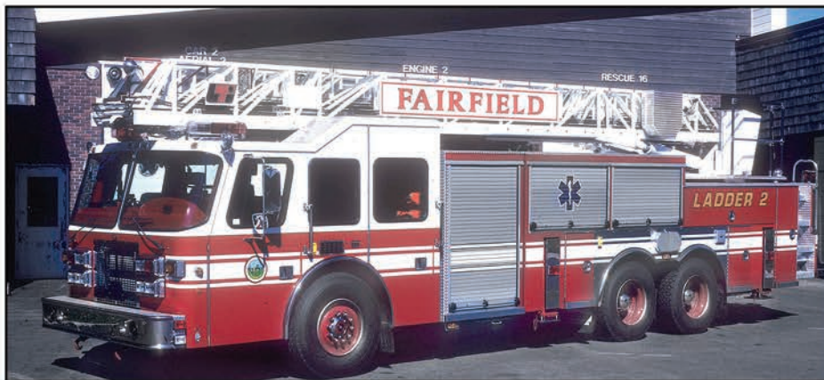
Fairfield, Connecticut, operated this 1995 Saulsbury rear-mount aerial ladder that was built on a Duplex chassis with a 100-foot LTI aerial ladder. Fairfield also operated a 1987 Saulsbury rescue, and a pair of 1995 Saulsbury pumpers.
