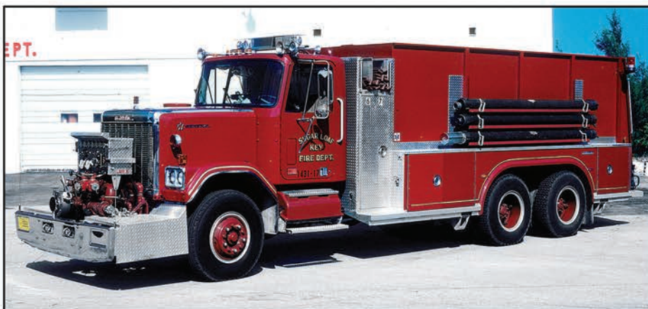
Sugarloaf Key in Florida was protected by this massive 1981 Saulsbury tanker-pumper that was built on a GMC General tandem axle chassis. This had a 1,000-gpm front mounted pump and a 3,000-gwt.
