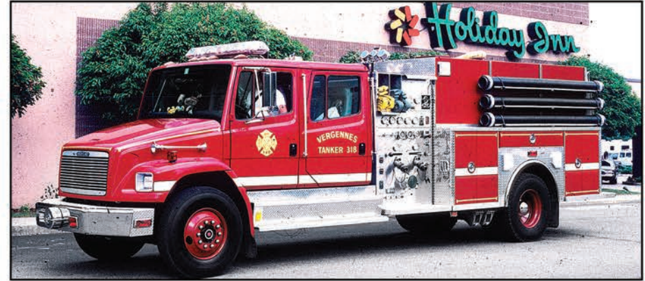
Built in 1994 with a 1,500-gpm pump and a 1,500-gwt, on a Freightliner chassis, this unit seems to straddle the line between pumper-tanker and tanker-pumper. To the uninformed, this might appear to be just a triple combination pumper. It still serves the fire department in Vergennes, Vermont, where it is identified as a tanker.
