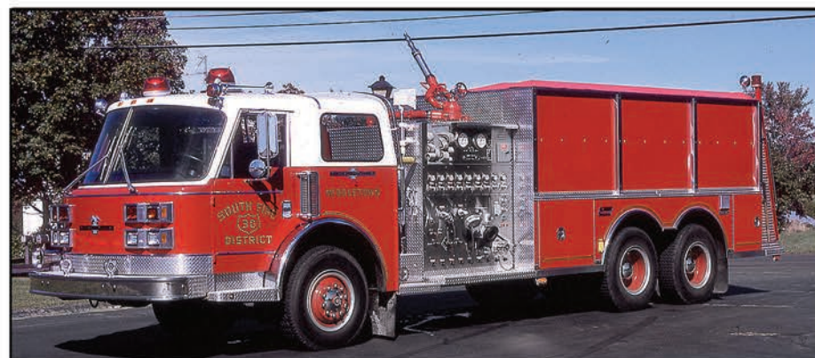
Saulsbury built this one-off pumper-tanker on a 1988 American LaFrance Century 2000 chassis. It served in Middletown, Connecticut, and had a 1,250-gpm pump and a 2,000-gwt. The Century 2000 was built in Bluefield, Virginia, by American LaFrance after the company was resurrected after closing its New York factory in 1985.
