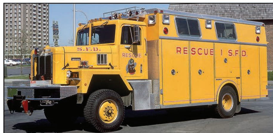
Among the most impressive rescue trucks built by Saulsbury was this one that was built in 1977 for Syracuse, New York, on an all-wheel drive International Paystar 5000 chassis. Its 18-foot body had access to the cab. It had 17 Kw generator and a 20,000 lb. capacity winch.
