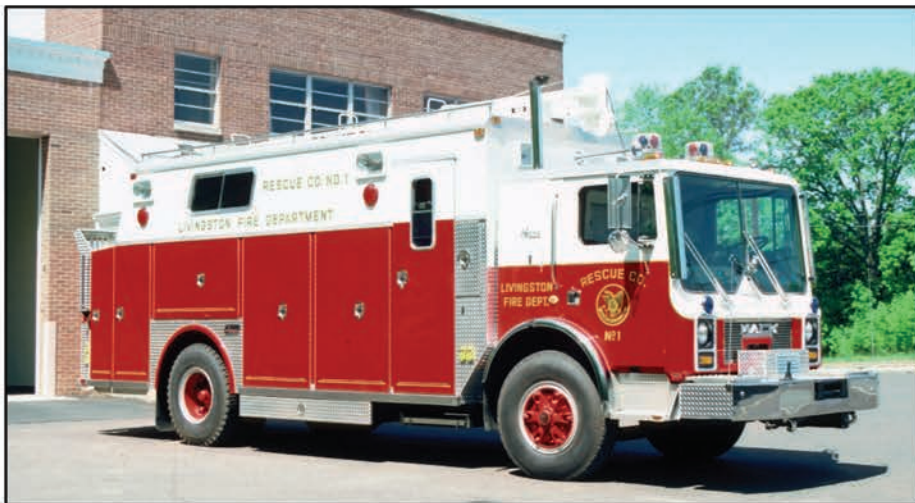
Livingston, New Jersey, operated this 1987 Saulsbury heavy rescue that was built on a Mack MC chassis and featured a rear mounted crane.
