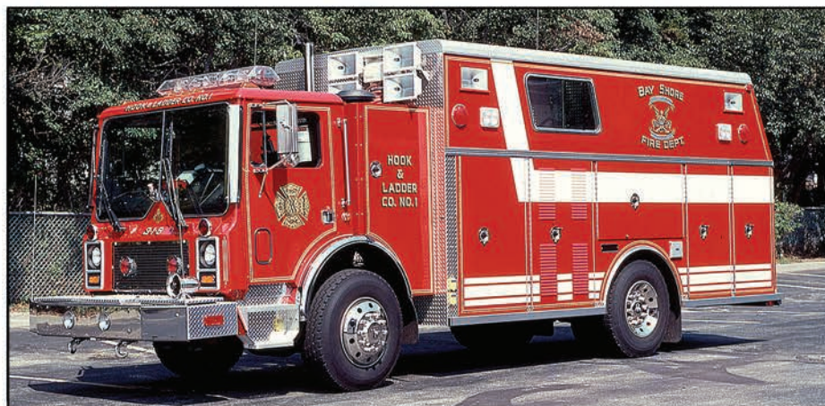
The Fire Department in Bay Shore, Suffolk County, New York, operated this 1990 Saulsbury walk-in heavy rescue built on a Mack MC chassis. The last fire apparatus to be built on the Mack MC chassis was another 1990 rescue truck, which Saulsbury built for Westbury, New York. 13
