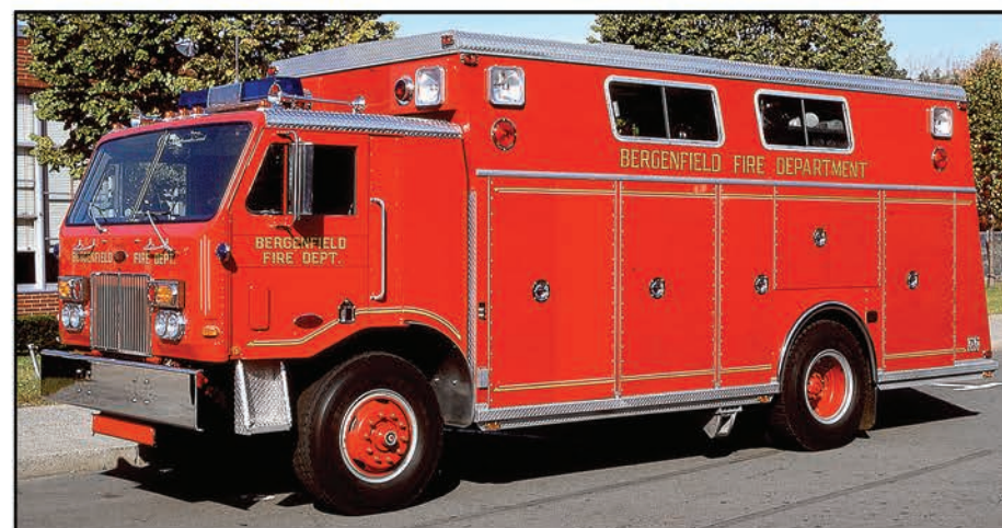
In 1977 the fire department in Bergenfield, New Jersey, had Saulsbury build this walk-in rescue truck on a Peterbilt Model CB300 cab-over engine chassis. The Peterbilt Model CB300 chassis was designed for refuse trucks and was a very unusual choice for fire apparatus.
