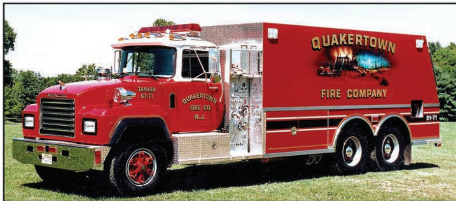
The flat sides of this 1992 Saulsbury 3000-gallon tanker provided a large canvas for a mural of a historic fire. This unit was built on a Mack RD chassis and had a 450-gpm pump. It also carried a 1,500-gallon folding tank. As the mural says, it serves in Quakertown, New Jersey.
