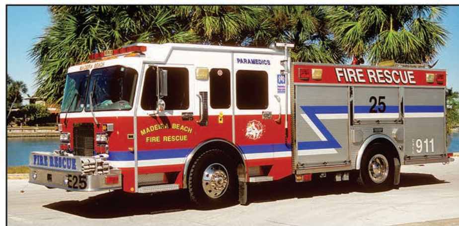
As the fire service began to perform much more emergency medical services than actual firefighting, Saulsbury started to build paramedic pumpers like this 1999 example that was built on a Spartan chassis with a 1,250-gpm pump, 500-gwt. and ample EMS compartments.
