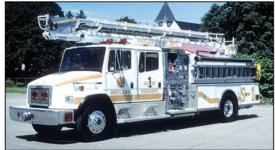
The Wayland Fire Department, in Steuben County, New York, operated this no-frills aerial unit. Squirt 1 was built on a Freightliner chassis with a 1,500-gpm pump, a 1,000-gwt. and a 50-foot Tele-Squirt aerial device.
