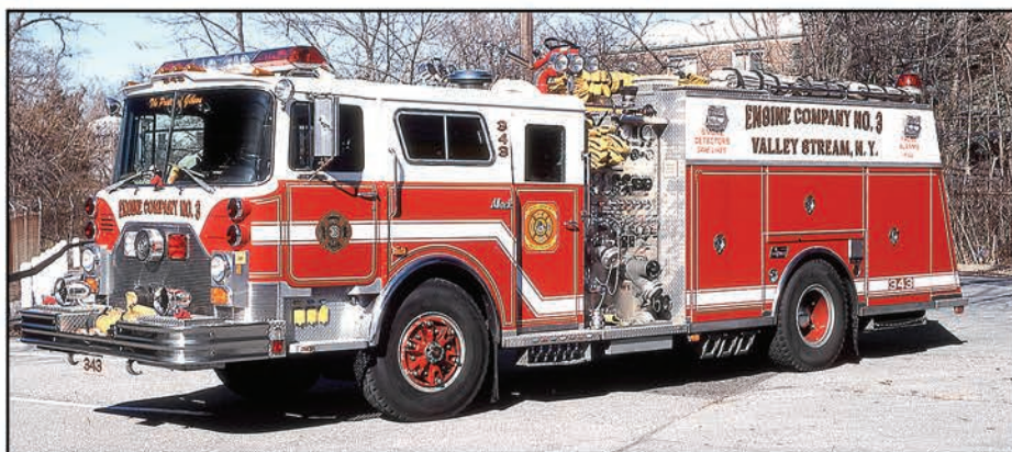
Responding as Engine 343 in Valley Stream, Nassau County, New York was this Mack CF pumper built by Saulsbury in 1988 with a 1,500-gpm pump and a 400-gwt. The pumper also carried 100 gallons of foam.
