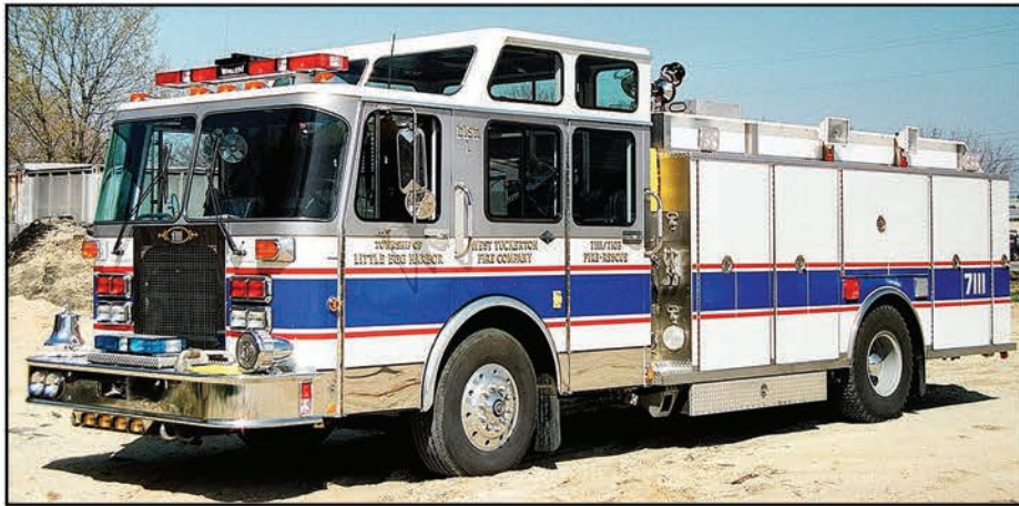
This 1990 Saulsbury rescue pumper looks more like a rescue truck than a triple combination pumper. It served in Little Egg Harbor, New Jersey. It had a 1,500-gpm pump and a 1,000-gwt.
