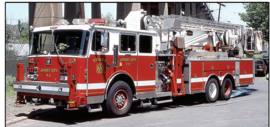
Jersey City, New Jersey, operated this Saulsbury tower ladder that was built on a tandem-axle Simon Duplex chassis with a 95-foot Baker Aerialscope. John Floyd photo.
