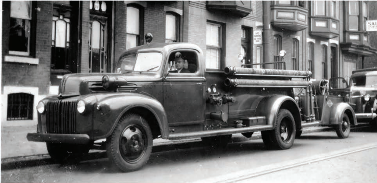
Unknown fire department with 500-gpm Ford pumper and unknown make trailer pump. Charles Beckwith Collection courtesy of Robert Lloyd.
