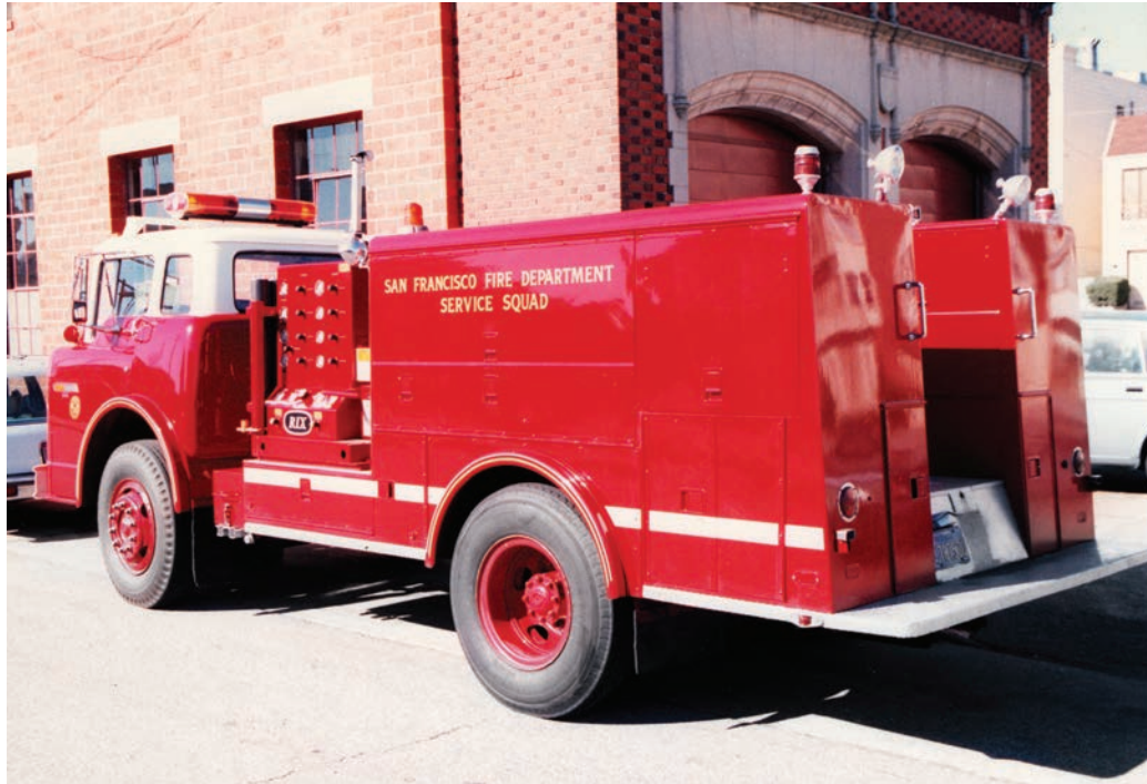
In 1982 a service squad body and air cascade body was installed on new chassis, a 1981 Ford C. In 1989 the air cascade system was replaced by a Rix air compressor for on-scene refilling.
