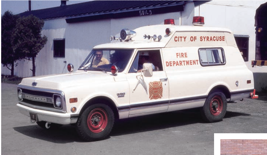
This 1970 Chevrolet C-20 Gerstenslager rig was the second generation of the First Aid unit and featured twin Dietz beacons on the roof along with a Federal mechanical siren. This rig would be replaced in the future with a series of modular ambulance bodies built by Medicoach, Modulance and Braun. Photo by Jack Calderone.
