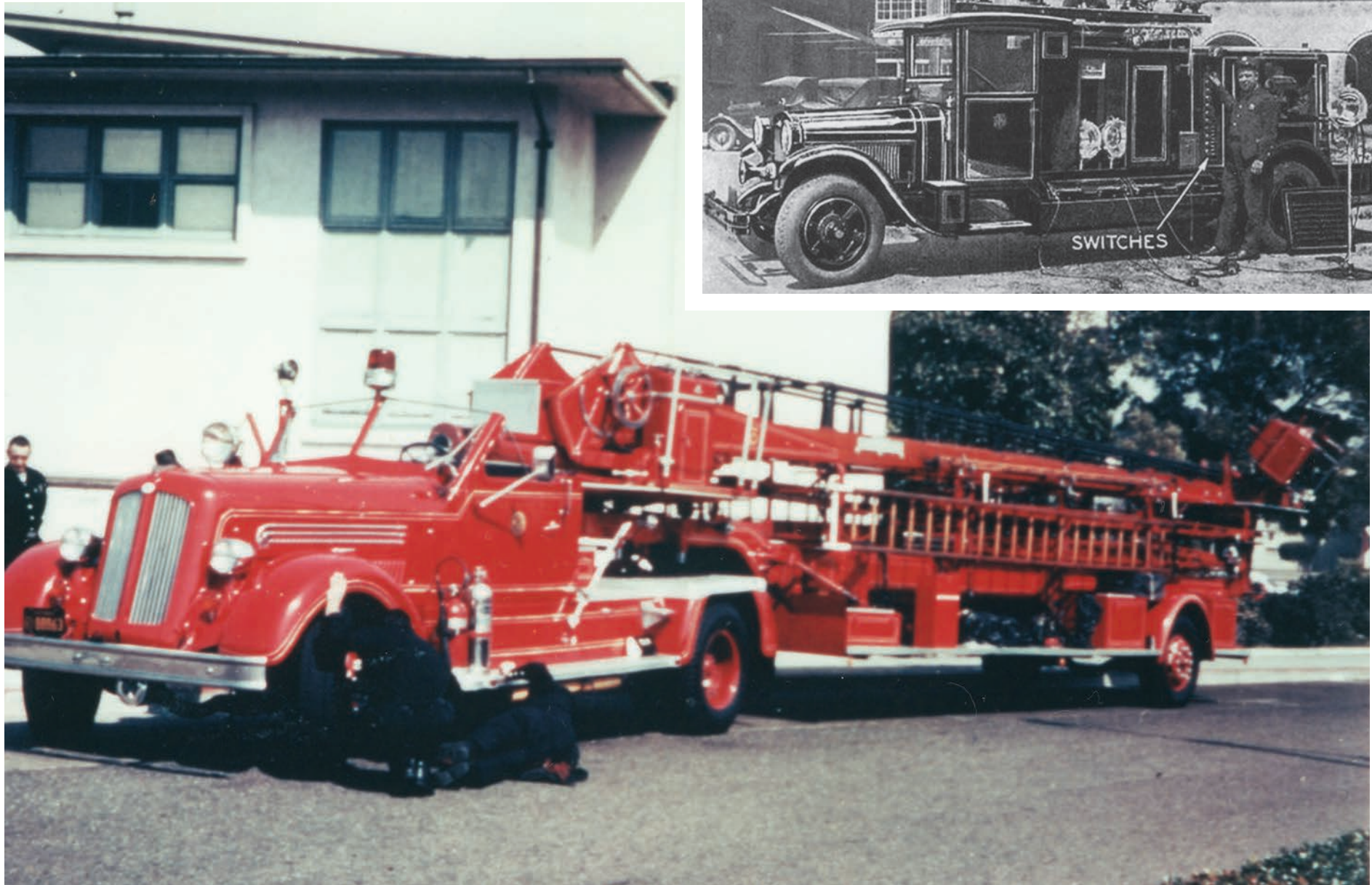
One of the two 1950 Seagrave tank that became ladder truck tractors with a 1939 Ahrens-Fox 85-foot wooden aerial ladder trailer.
