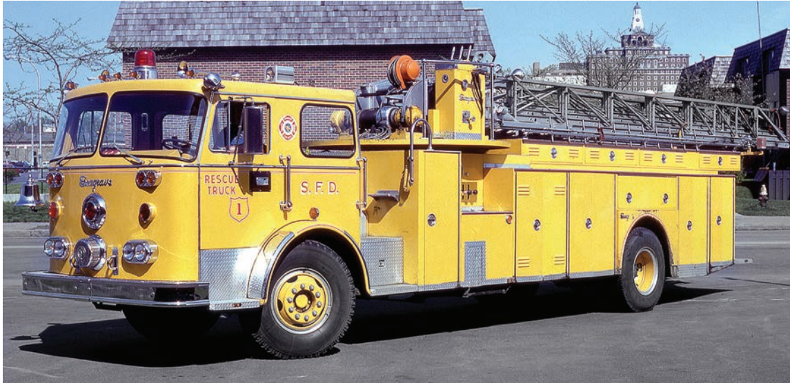
This 1973 Seagrave PA-20756 100 foot midship aerial ladder first served as Truck 2 and reassigned to the Rescue Company in 1976. This rig was equipped with 268 feet of ground ladders, including a scaling ladder mounted above the upper body compartments. Photo by the late Pete Lund.
