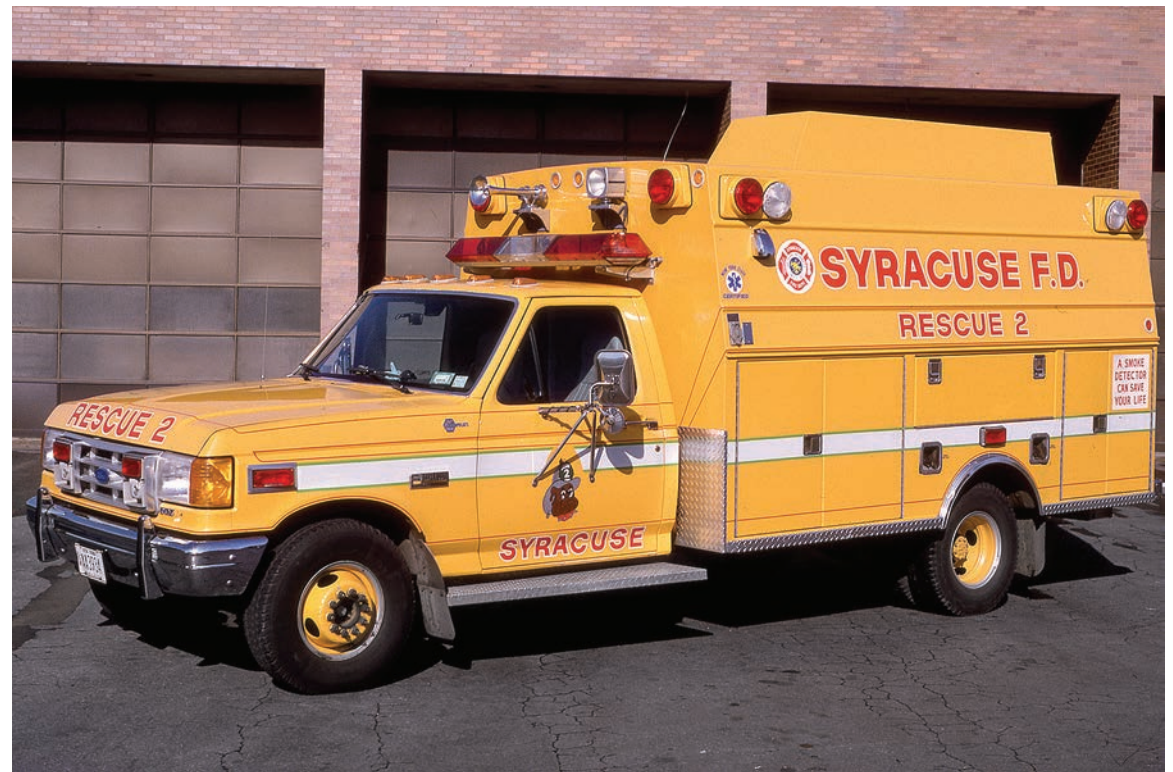
Rescue Two operated with this 1992 Ford F-250 chassis carrying a Braun model BF-3000A modular body with serial number 2088. The compartment on top of the body carried a stokes basket and backboards. Photo by Tom W. Shand.
