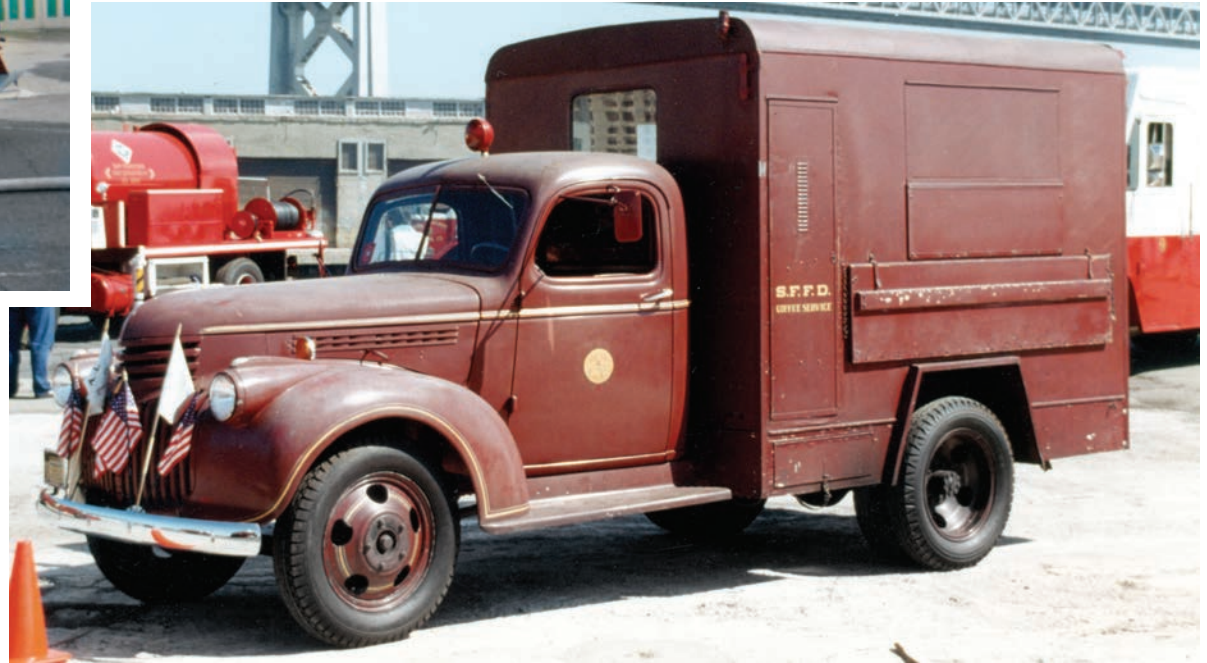
In 1946, a 1942 Chevrolet 1-1/2-ton chassis of a formerly Auxilliary Defense pumper received the shop-built body from a 1922 Buick to become the new "Coffee Wagon."
