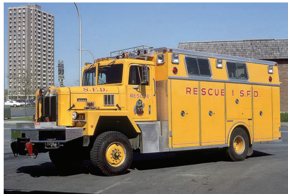
Syracuse Rescue One operated this 1977 International Paystar 5070 4X4 chassis with bodywork built by Saulsbury Fire Equipment. This rig defines the term Heavy Rescue and was the first walk through style body built by Saulsbury and equipped with a 17.0Kw direct drive generator, and A-Frame with a 20,000-pound hydraulic front winch. Photo by the late Pete Lund.
