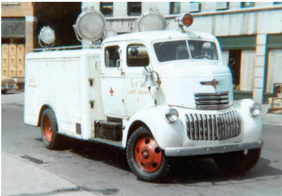
The Light Squad operated this 1941 Chevrolet four door cab chassis with custom bodywork built by the Salina Body Works enabling the company to carry additional equipment with a 5.0 Kw generator and floodlights. Photo from the collection of Tom W. Shand.
