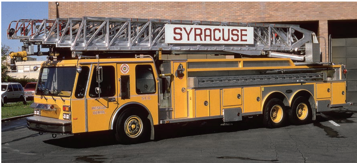
This 1985 Emergency One Hurricane 135-foot aerial ladder was acquired to enhance the capabilities of the Rescue Company. This rig was one of twenty seven 135 foot ladders built by Emergency One assigned serial number 3984 and cost $315,000 when new. Photo by Tom W. Shand.
