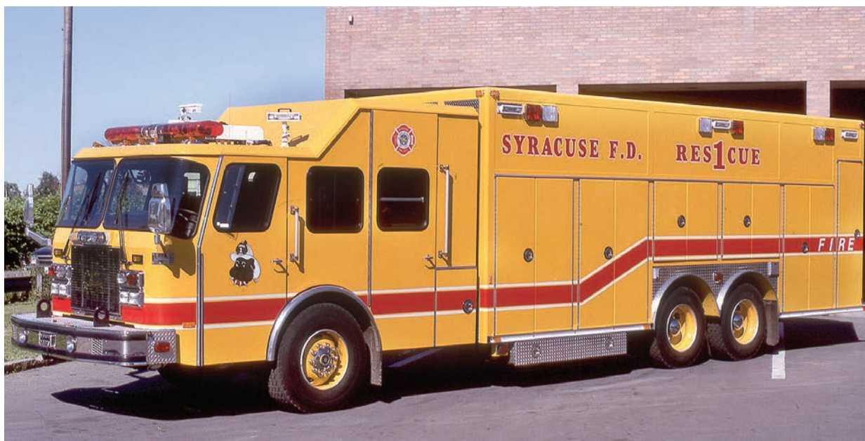
This 1997 Emergency One Cyclone apparatus was one of the last to enter the departments fleet in the chrome yellow color. Serial 17764 was built on a 246-inch wheelbase with a twenty five foot aluminum walk in body equipped with a 35 Kw Onan direct drive generator. In later years, the apparatus was repainted red to match the department's new paint scheme. Photo by Tom W. Shand.
