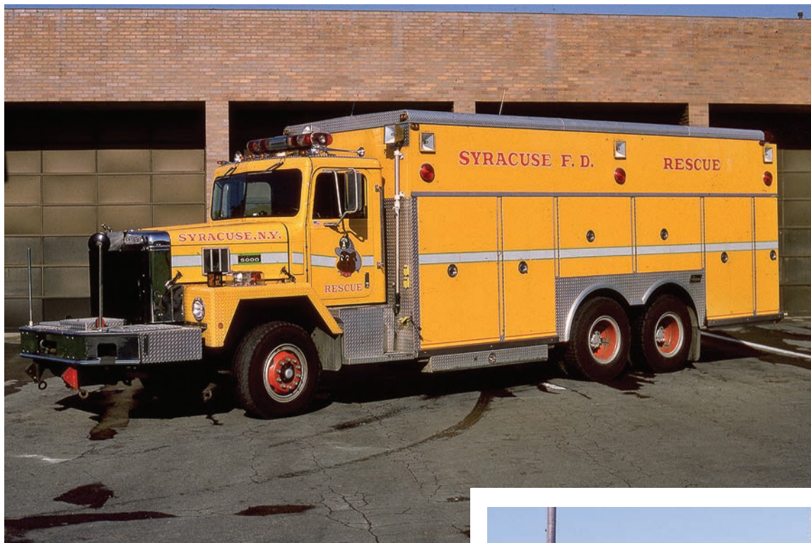
The Rescue Companies first tandem axle apparatus was this 1986 International Paystar 5070 chassis powered by a Detroit Diesel 8V-92TA engine rated at 450 horsepower on a 212-inch wheelbase built by Saulsbury Fire Equipment. The stainless steel body had a walk through from the cab and was equipped with a 17.0 Kw direct drive generator and carried Saulsbury serial number 2456. Photo by Tom W. Shand.
