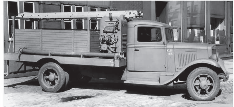
Hale pump package on a flat-bed truck of the Cleveland Auxiliary Fire Department for illustration of pump package. Photo from the Paul Nelson Collection.
