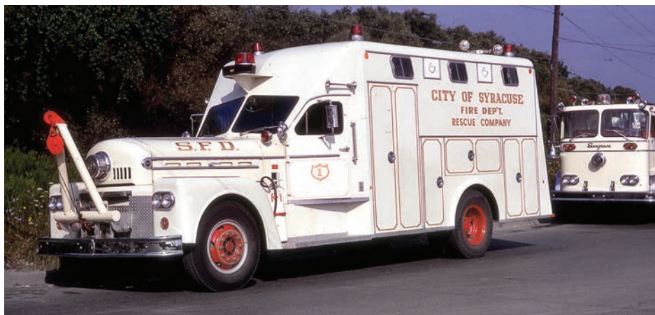
This classic 1966 Seagrave 70th Anniversary model rescue was built by Welch Fire Apparatus in Marion, Wisconsin. Seagrave supplied the chassis with the open cab and cowl with Welch mating the cab roof and bodywork with a streamlined appearance. This rig was powered by a Waukesha F-817G engine rated at 325 horsepower, with the Fire Department shops adding the front bumper winch and A-frame, assigned Seagrave serial number Q-4066. Photo by Jack Calderone.
