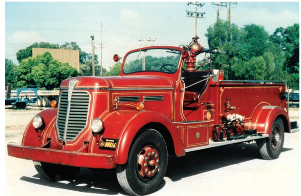
One of the two 1940 Fabco tank wagons that were converted into Hose Tenders with Gorter turrets between 1958 and 1960.
