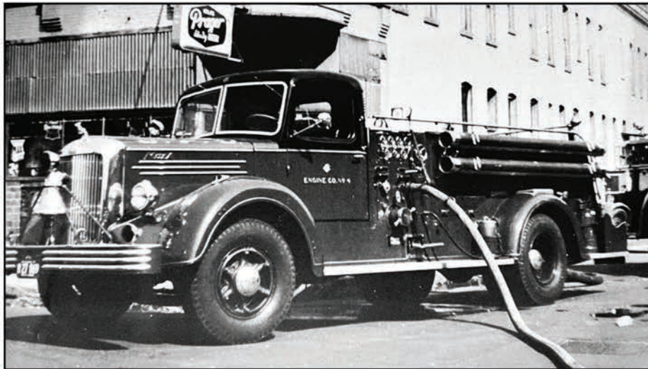
In 1949 Chicago modernized its aging fleet with 32 Type L-95 pumps with coupe cabs and 1000-gpm pumps.
