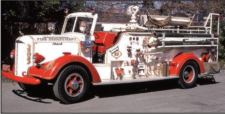
During World War Two, the port of Baltimore was one of the busiest and most important. The Baltimore Fire Department operated this 1944 doorless L-80 750-gpm pumper.
