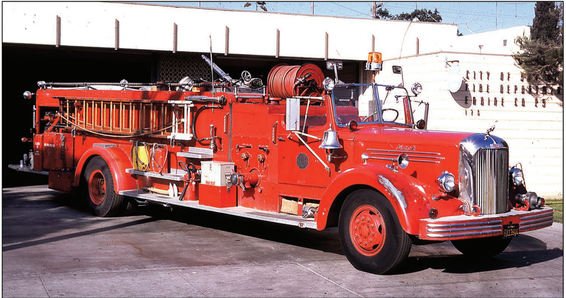
The rugged L Model Mack was well-suited to demands imposed by fire service. This 1947 Type L-95 quadruple combination served in San Diego, California. With everything from a booster reel to a deck pipe as well as a 1000-gpm pump and variety of ground ladders, this truck was extremely well-equipped. Note the short length of supply line located under the officer's door and the shovel under the running board just ahead of the rear wheels.
