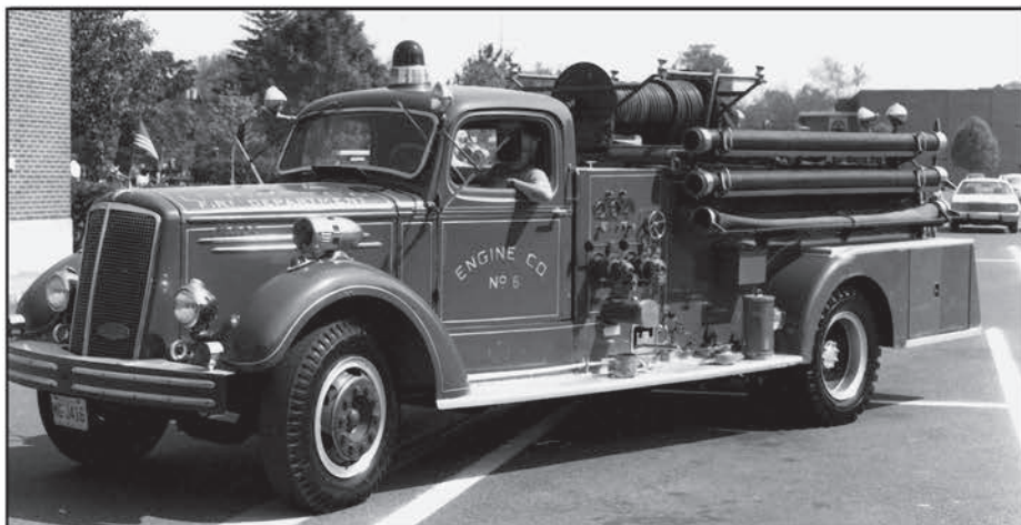
Post-war deliveries of Mack fire apparatus made in Long Island City included this 1948 L-85 pumper, above, for the Brooklyn Fire Company in Anne Arundel County, Maryland, and this 1949 Type 505S, below, for Livingston, New Jersey. Note the rear fender compartments.
