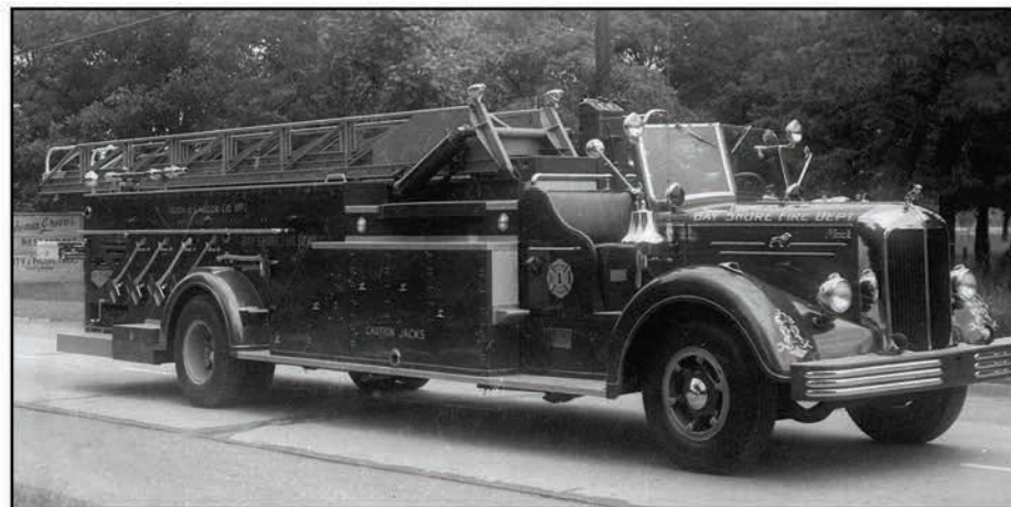
Above: This 1951 Mack Type 75LS service aerial ladder served in Bayshore, Long Island, New York. Note the quintet of axes mounted behind the rear fender.
