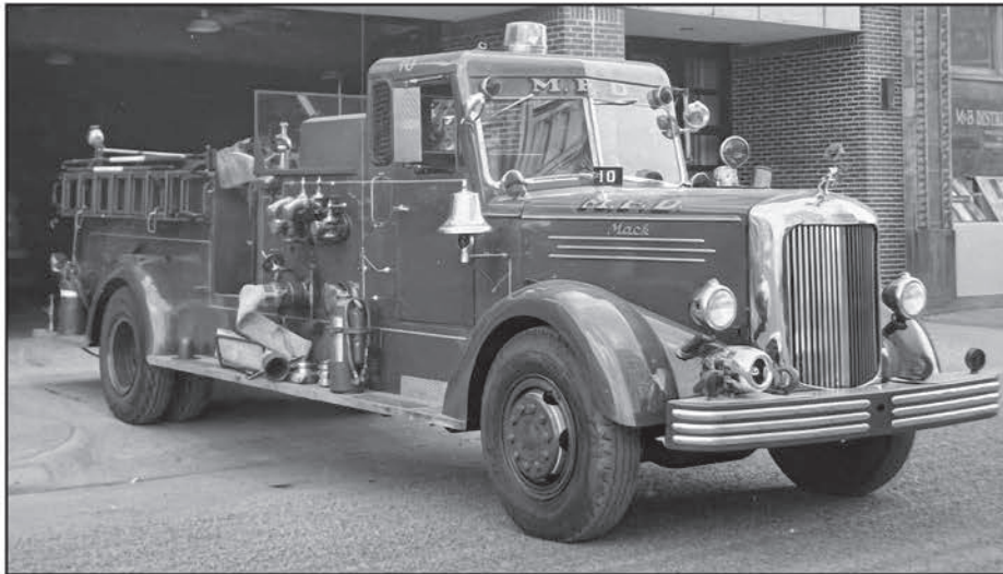
Some superlative Macks were made in New York, including several for Minneapolis, Minnesota, which are seen here in photos by the late Dan Martin. The first were a pair of 1948 Type 21 pumpers that were built with 2000-gpm Waterous pumps. In 1962 these had their cabs enclosed.
