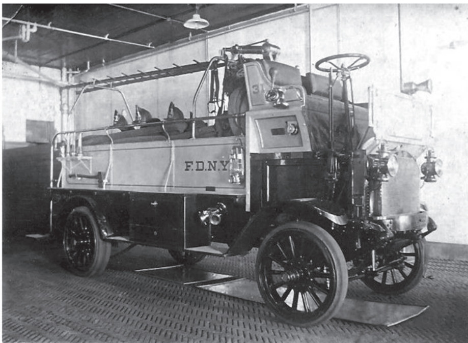
This is one of three 1912 high pressure hose wagons that were built on a heavy-duty Mack Senior chassis with bodies by James Boyd and Brother of Philadelphia.
