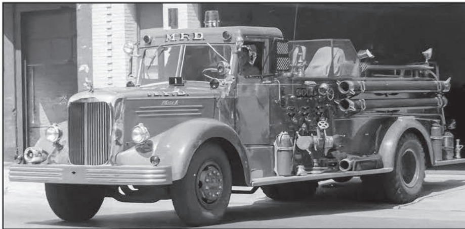
In 1949, Minneapolis purchased this Type 21 pumper with a 1500-gpm Hale pump.
