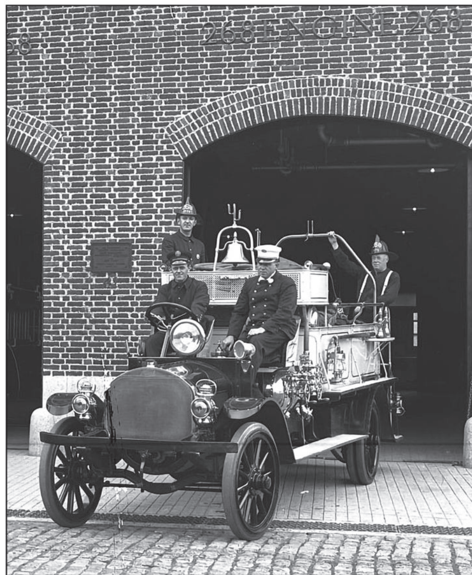
When FDNY Engine Company 268 was formed in 1912, it was assigned to a new station that was built specifically for motor fire apparatus. The company was assigned this new double tank chemical engine and hose wagon combination that was built on a Mack Junior chassis.
