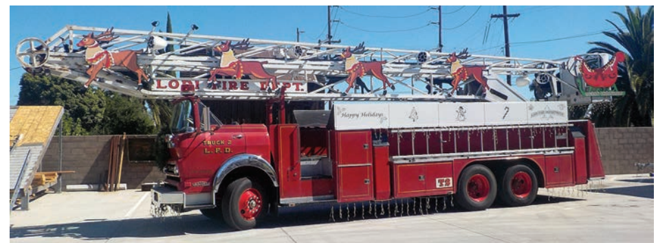
Lodi (CA) Fire Department keeps a "Santa fire truck" in their firehouse. The "snorkel basket" on their 1967 GMC/Van Pelt/Hi-Ranger is permanently decorated as Santa's sleigh, with reindeer lining both sides of the "snorkel" boom. The 85-foot cable-hoist raise mechanism has been disabled, and a more modern diesel engine and automatic transmission have been installed.
