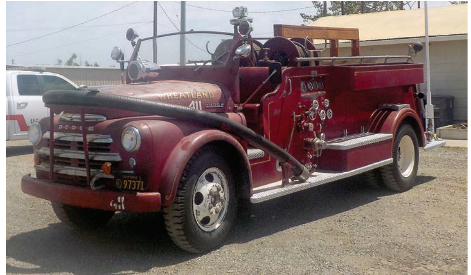
Wheatland (CA) still owns this 1949 Dodge/Van Pelt pumper. The Dodge has a 500-gpm pump and 500-gwt. All photos by Ed Hass.
