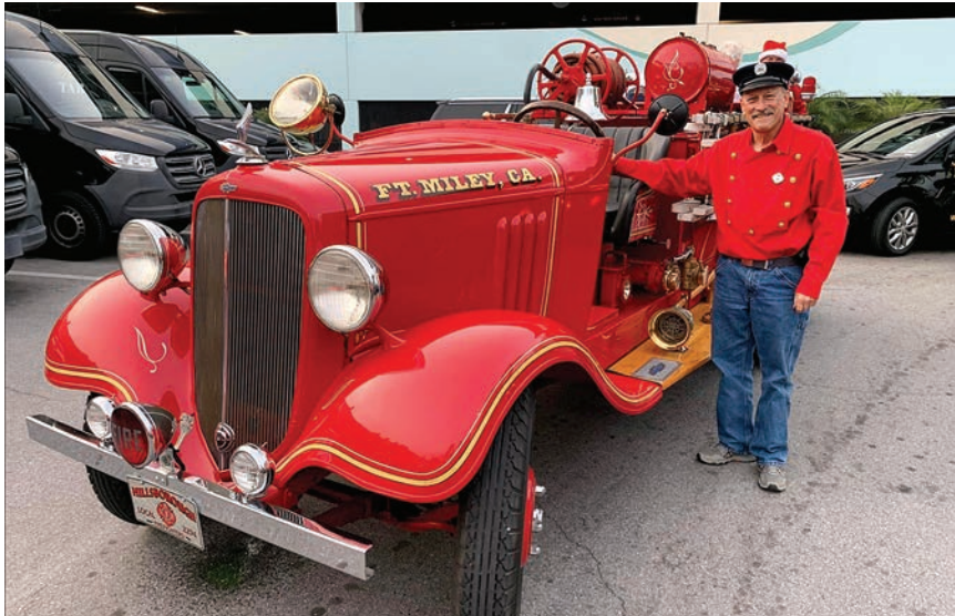
Doug Riddle's 1934 Chevrolet/Howe pumper (ex-Veterans Administration for Fort Miley Veterans Hospital, San Francisco, CA). The Howe is a triple combination pumper mounted on a 1 1/2 ton chassis. Basic specifications include a 200-gwt, 12-gauge copper baffled booster tank, and a 200-gpm Waterous Rotary gear pump.
