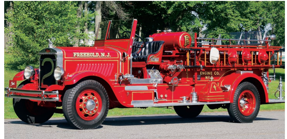
1930 Mack BX pumper (ex-Freehold, NJ). The rig has a 750-gpm pump.
