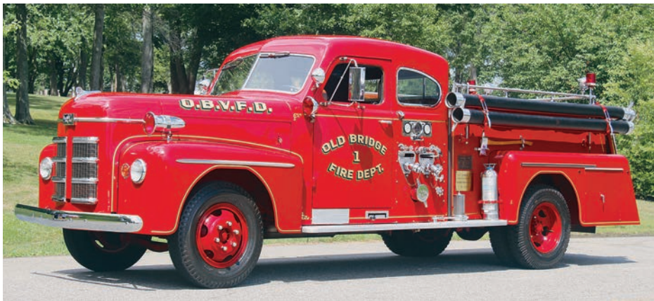
1947 Ahrens-Fox pumper (ex- Old Bridge Fire District, East Brunswick, NJ) that was refurbished by Hahn in 1988. The Fox has a 750-gpm pump and 200-gwt.
