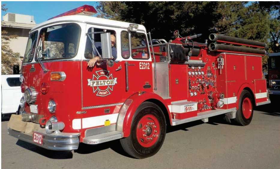
Mark Hathaway's 1966 Crown Firecoach pumper (ex-Live Oak, CA and ex-Felton, CA). The Crown has a 1,250-gpm pump and 500-gwt.
