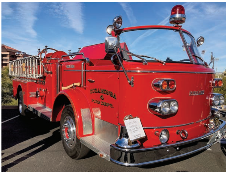
1968 E. R. Foden/ Hampshire Car Body Angus Pump Escape. Angus built over 6,500 pieces of fire apparatus during its 61 years of existence between 1933 and 1994. This rig was built for Nottinghamshire (U.K.). It has a rear mount 750-gpm pump (with engineer panels on both sides of the truck).
