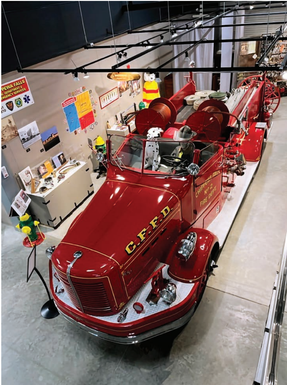
Wheatland (CA) still owns this 1949 Dodge/Van Pelt pumper. The Dodge has a 500-gpm pump and 500-gwt. All photos by Ed Hass.
