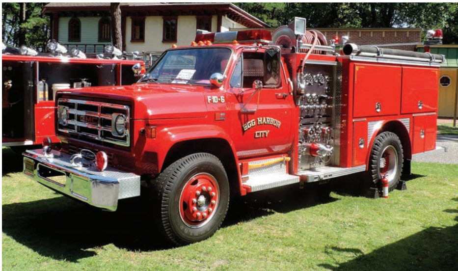
William Sorshek's 1983 GMC/Emergency One pumper looks as it did on delivery day to the Egg Harbor City (NJ) Fire Department. This unit has a 1,000-gpm pump and 500-gwt.
