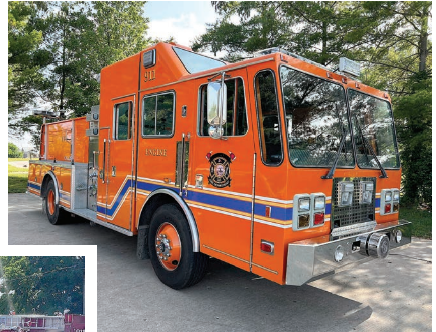
1991 KME Predator pumper (ex-Fortville, IN) has a 1,250-gpm pump and a 750 gwt. The KME is unique with its extra tall cab that enclosed the mid-mount pump panel. The KME is part of the Ted Moore Collection.
