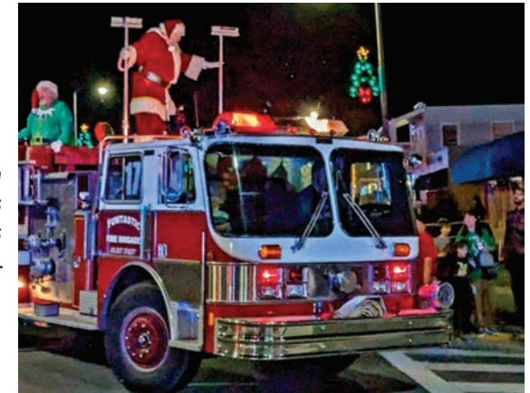
Steve Vinson owns this 1989 Spartan Diamond/FMC pumper (ex-Kenansville, NC). The FMC has a 1,250-gpm pump and a 1,000-gwt.
