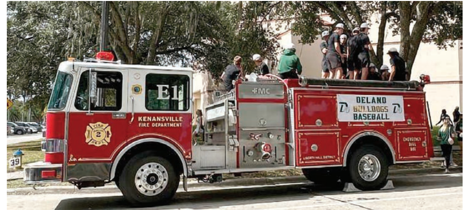
Steve Vinson owns this 1989 Spartan Diamond/FMC pumper (ex-Kenansville, NC). The FMC has a 1,250-gpm pump and a 1,000-gwt.
