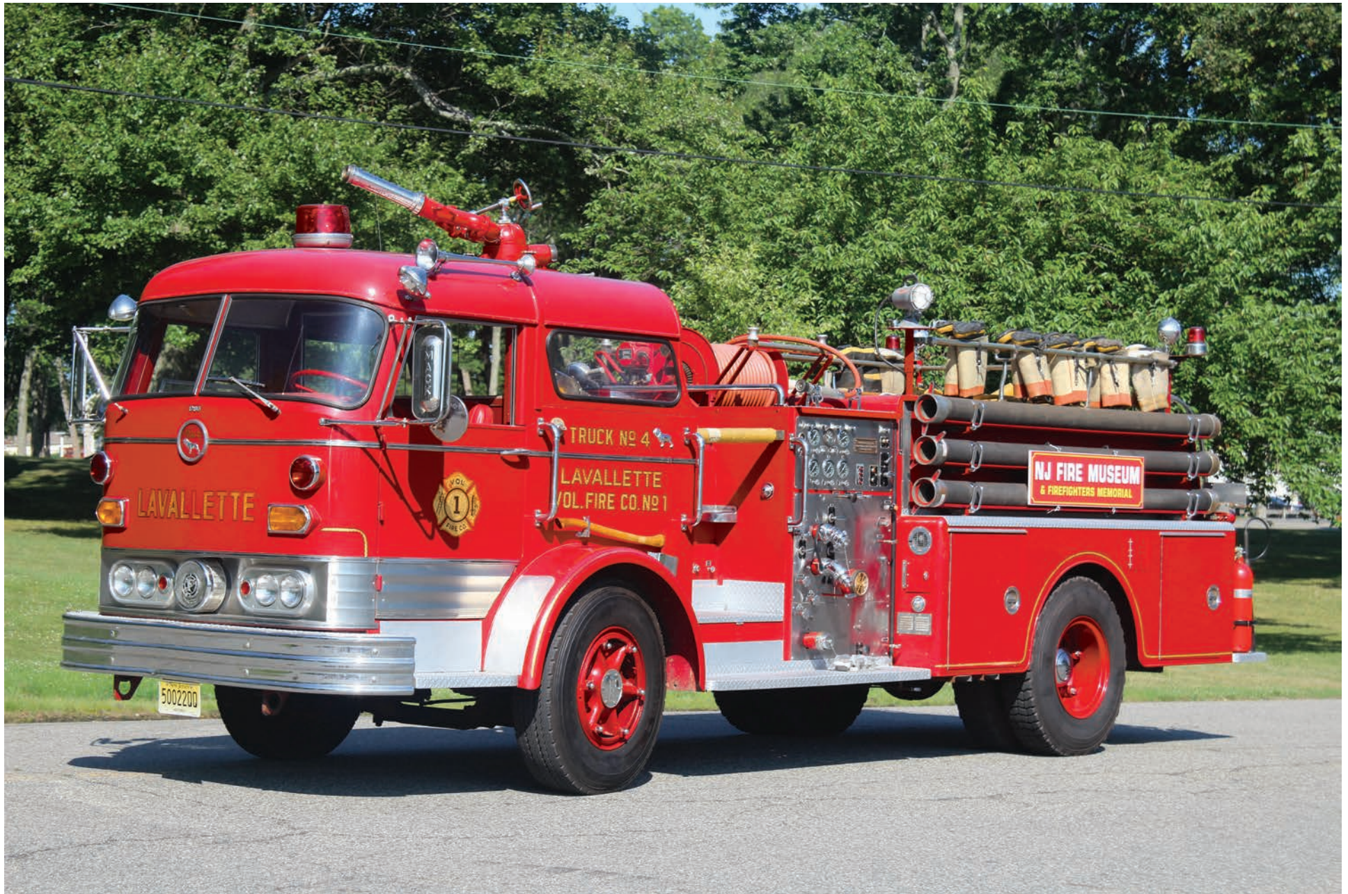
1967 Mack C pumper (ex-Lavallette, NJ) is equipped with a 750-gpm pump and 500-gwt. The Mack is part of the New Jersey Fire Museum Collection.
