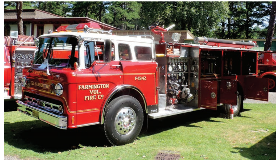
1986 Ford C/Pierce pumper (ex-Farmington Fire Company in Egg Harbor Township, NJ) is also owned by William Sorshek. The pumper has a 1,250-gpm pump and 1,000-gwt.
