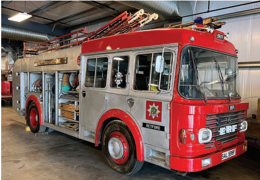
1968 E. R. Foden/ Hampshire Car Body Angus Pump Escape. Angus built over 6,500 pieces of fire apparatus during its 61 years of existence between 1933 and 1994. This rig was built for Nottinghamshire (U.K.). It has a rear mount 750-gpm pump (with engineer panels on both sides of the truck).
