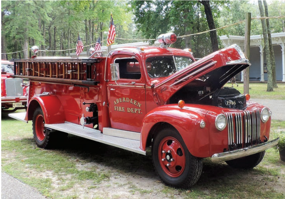
This 1946 Ford/Oren pumper (ex-Aberdeen (MD) Fire Department) is equipped with a 500-gpm pump. The Ford is owned by the Piper family.
