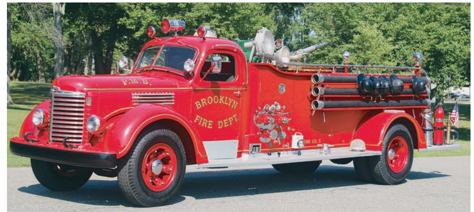
1947 International/Great Eastern pumper (ex-Hampton, NJ) has a 500-gpm pump and 300-gwt.
