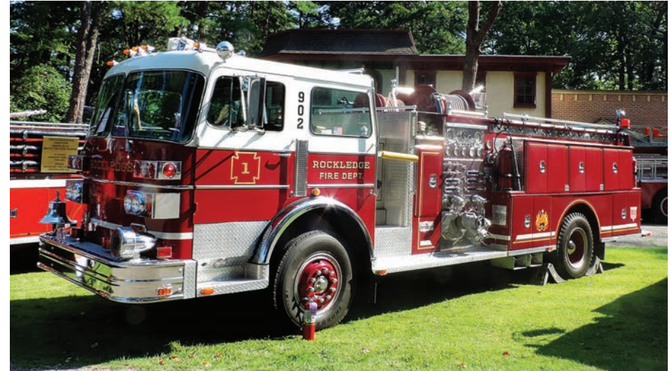
William Foxall Jr. displayed this 1981 Sutphen pumper (ex-Rockledge PA) which had served his department for many years. The pumper has a 1,250-gpm pump and 500-gwt. The Sutphen was ordered by Rockledge in 1979, completed in December 1980, and registered in 1981.
