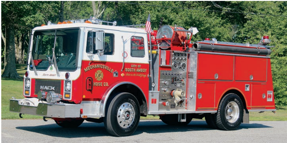
Part of the New Jersey Fire Museum Collection is this 1986 Mack/RSI pumper (ex-South Amboy, NJ). The Mack is equipped with a 1,250-gpm pump and 500-gwt.
