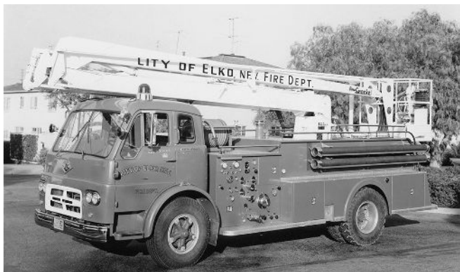
Crown's first Snorkel was this 750gpm/300 gallon/50' model built for Elko (NV) on an International chassis. Crown Coach photo by Warren Bowen from the CFE archives.
