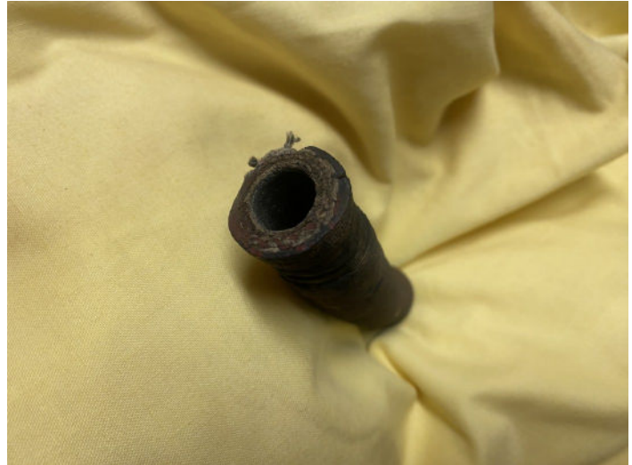
Vacuum Hose End Where it Connected to Pump
