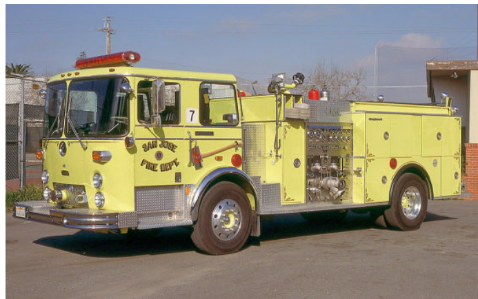
This is a Van Pelt pumper that used a Crown Firecoach Cab & Chassis (Crown Special Cab & Chassis job 75002). This was Van Pelt #830435 using an FMC steel Roughneck hosebed body. (Photo by Chuck Madderom from the Crown Firecoach Archives.
