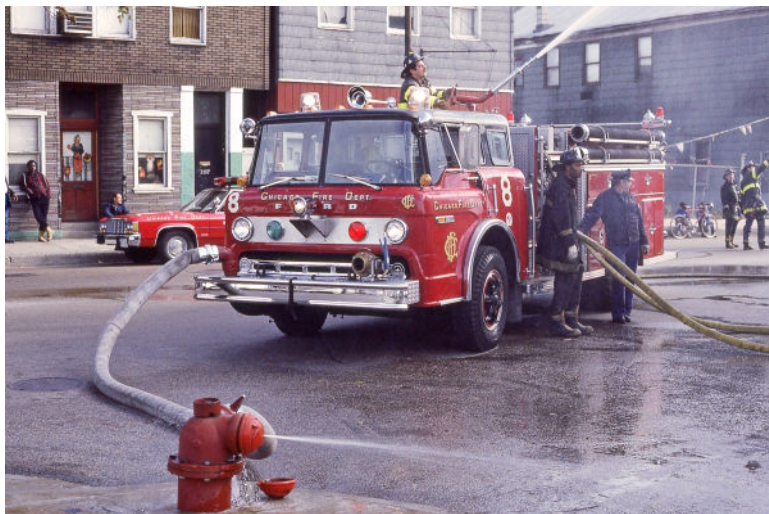
Left: This C model Ford/E-One is using a front suction port to supply its deck gun plus two hand lines. It has a Cat motor. Chuck Madderom photo
