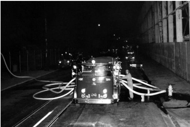
I have no idea what is going on here in Vernon (CA). The '57 Crown with a Hall Scott motor appears to have two lines off the hydrant feeding the pump. Chuck Madderom photo
