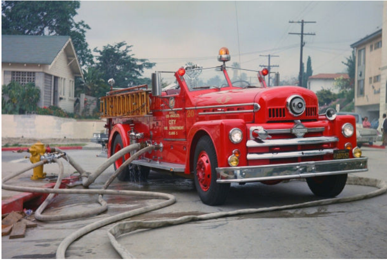
Left: This is an exotic hookup by a Los Angeles Seagrave with a Hall-Scott motor. It looks like three lines from the hydrant are being used. Chuck Madderom photo
