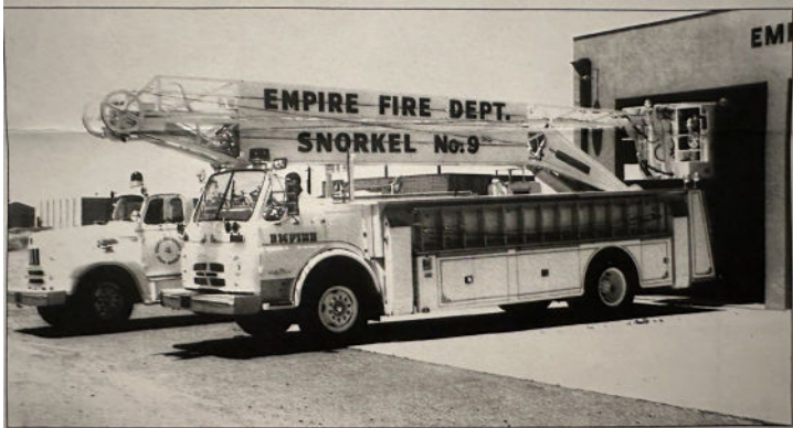
(above) Empire's 1966 International VCO-206/Van Pelt 65 ft Hi-Ranger articulating-boom aerial platform (s/n 618196) was the department's only aerial. Van Pelt installed Hi-Ranger aerials from 1961 to 1971. (Wayne Sorensen photo courtesy of the San Jose Fire Museum)
