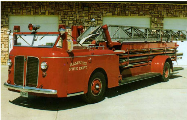
A "standard" JOX with its open ladder rack. Credit: Photographer
