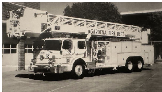
(above) Gardena's massive 1979 Duplex/Van Pelt 85 ft LTI telescoping-boom aerial platform had a 1500 gpm pump and 300 gal tank (s/n 727419). (Chuck Madderom photo)
